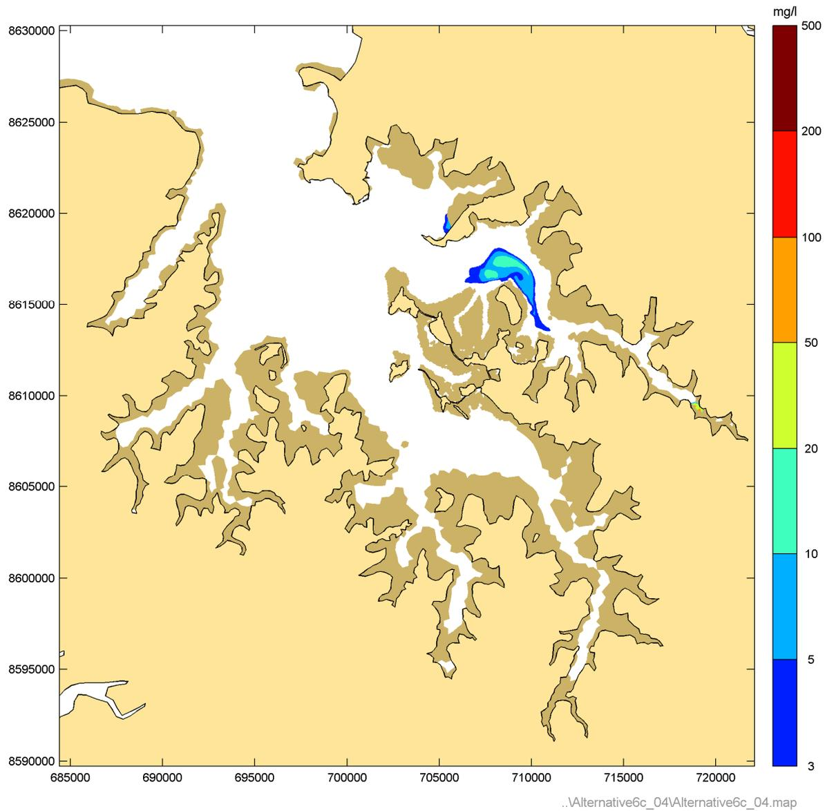
**Figure 53** Instantaneous suspended sediment concentrations during Phase 4 peak flood – Neap tide
