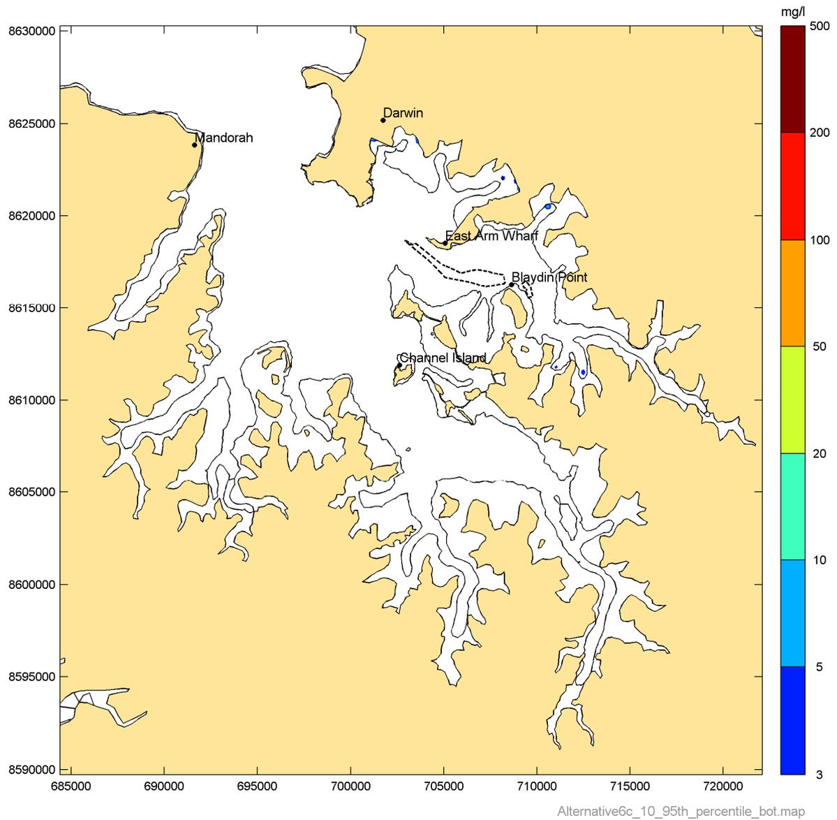
**Figure 39** Simulated 95<sup>th</sup> percentile suspended sediment concentration in the East Arm for Phase 10
