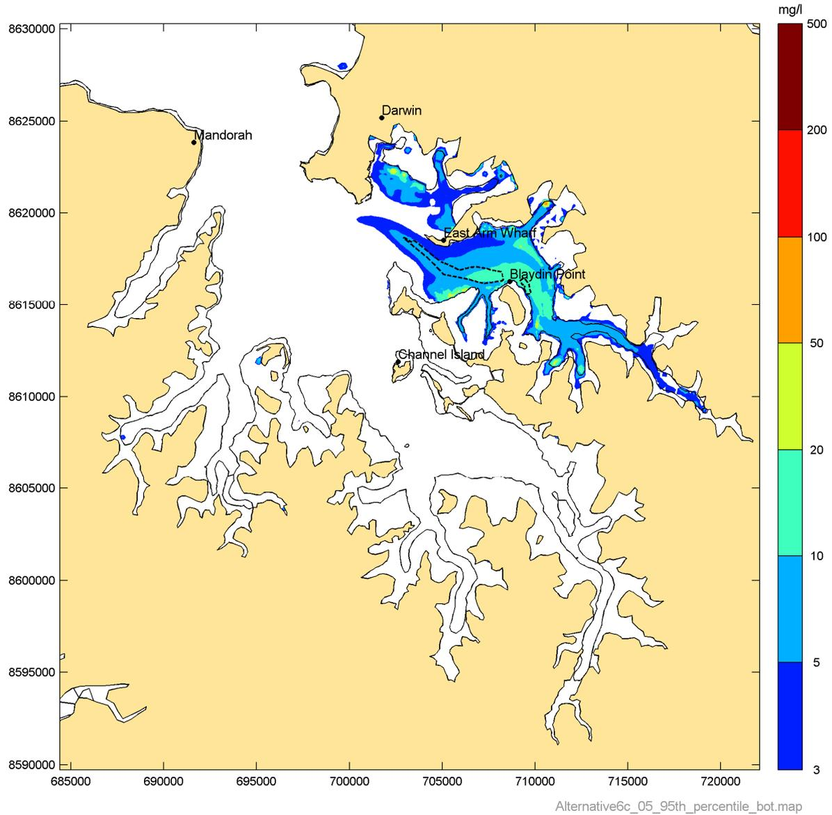
**Figure 33** Simulated 95<sup>th</sup> percentile suspended sediment concentration in the East Arm for Phase 5
