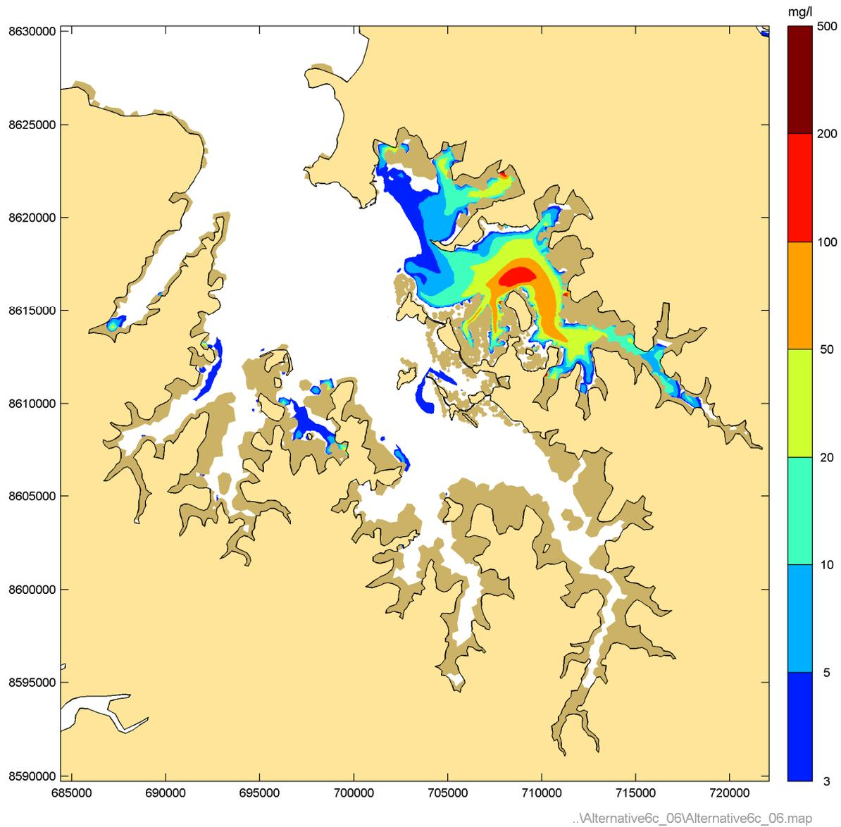
**Figure 67** Instantaneous suspended sediment concentrations during Phase 6 peak flood – Spring tide (cutter-suction dredger activity)
