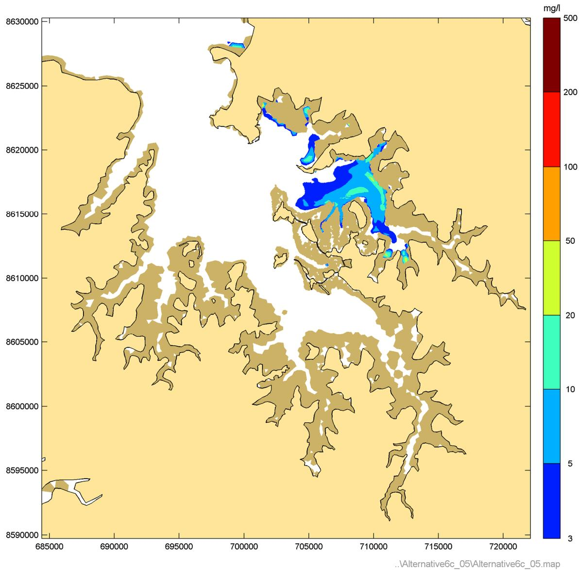
**Figure 59** Instantaneous suspended sediment concentrations during Phase 5 peak flood – Spring tide
