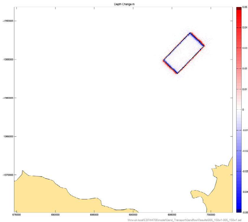
**Figure 150** Difference in potential area and magnitude of deposition and erosion at the proposed offshore disposal ground under tide plus wave conditions
