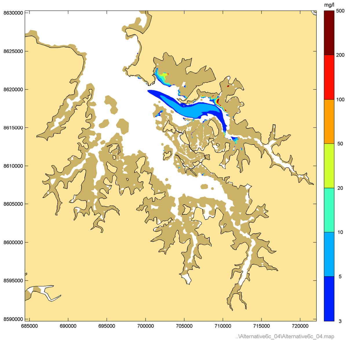
**Figure 54** Instantaneous suspended sediment concentrations during Phase 4 peak ebb – Spring tide
