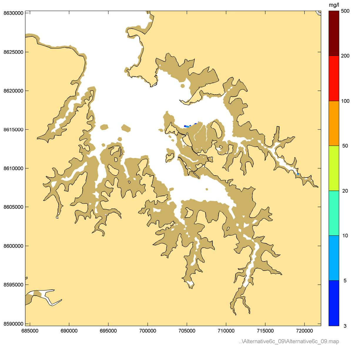
**Figure 76** Instantaneous suspended sediment concentrations during Phase 9 peak ebb – Neap tide
