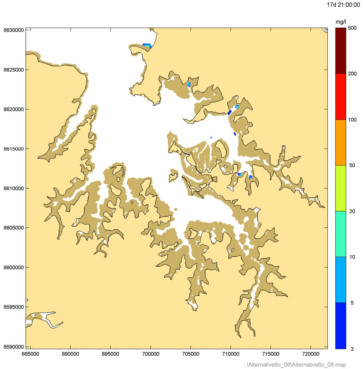
**Figure 75** Instantaneous suspended sediment concentrations during Phase 8 peak flood – Spring tide
