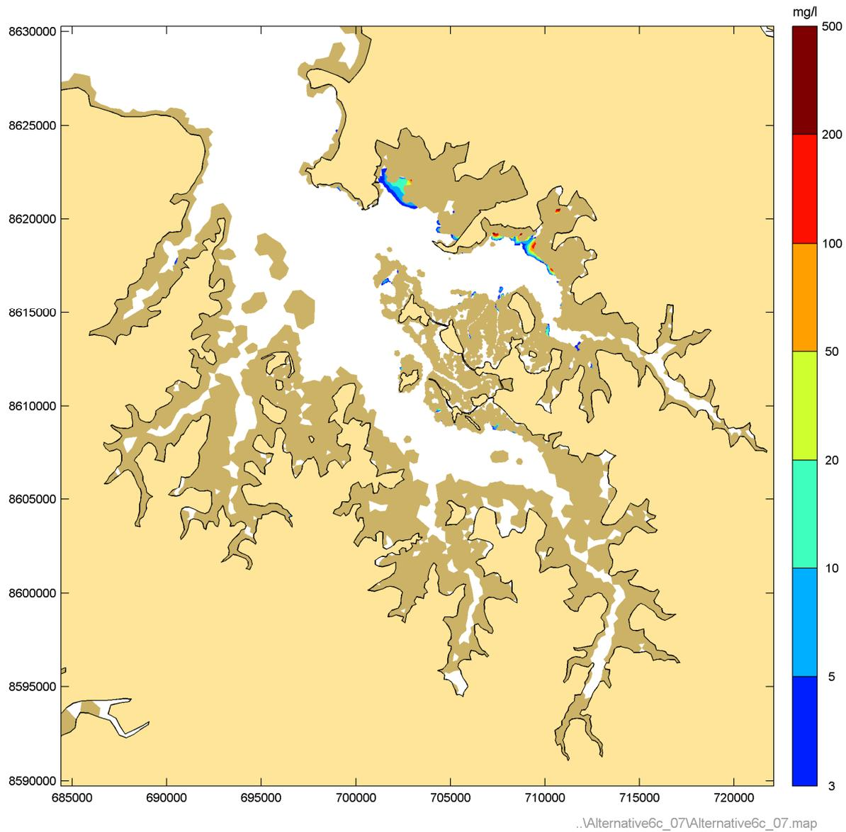
**Figure 70** Instantaneous suspended sediment concentrations during Phase 7 peak ebb – Spring tide
