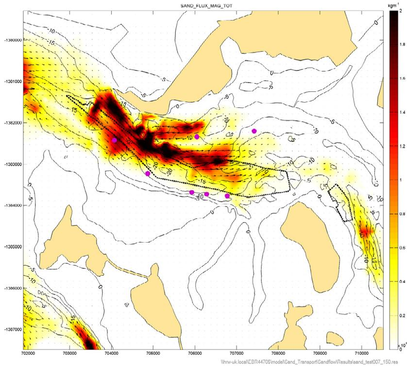
**Figure 130** Net sand transport for spring-neap cycle 150 µm sand under tide-only conditions for predredge bathymetry
