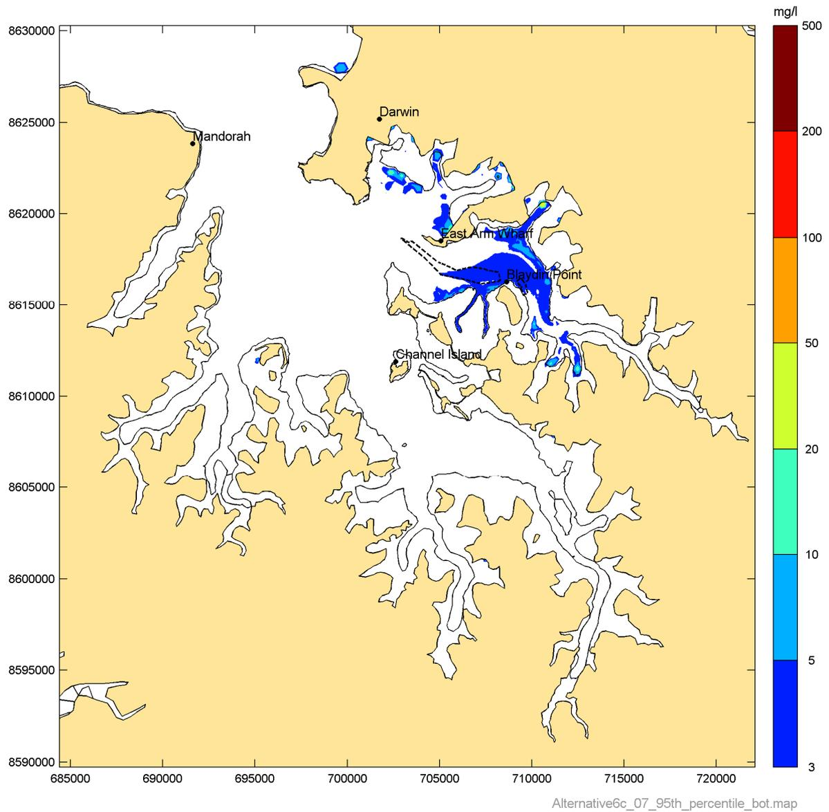
**Figure 36** Simulated 95<sup>th</sup> percentile suspended sediment concentration in the East Arm for Phase 7
