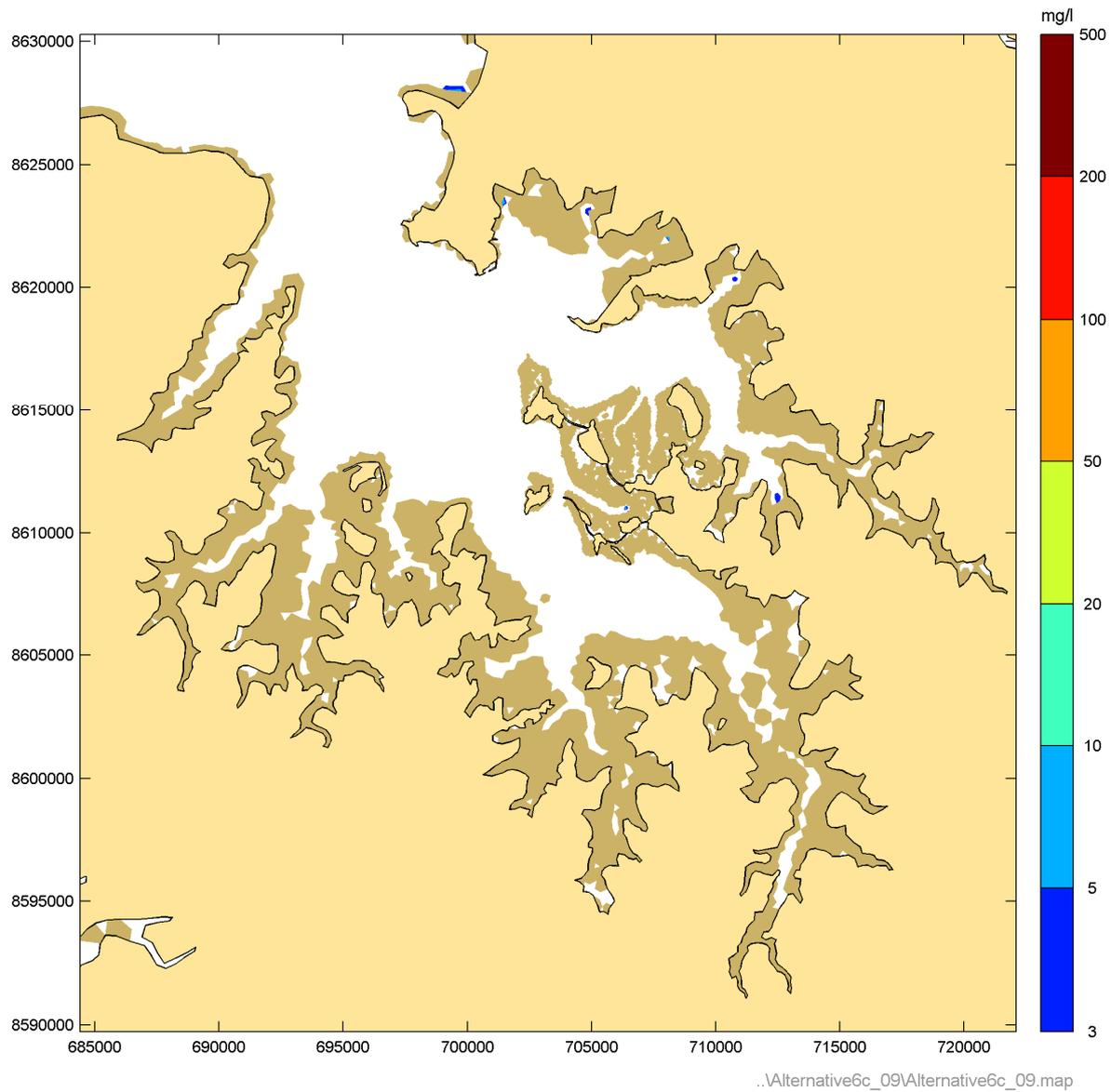
**Figure 79** Instantaneous suspended sediment concentrations during Phase 9 peak flood – Spring tide
