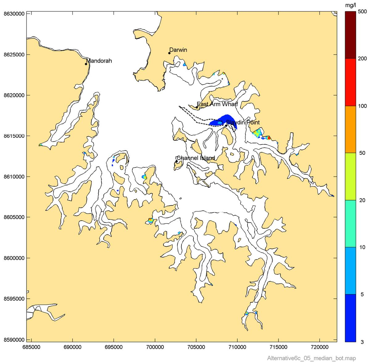
**Figure 22 Simulated median suspended sediment concentration in the East Arm for Phase 5**
