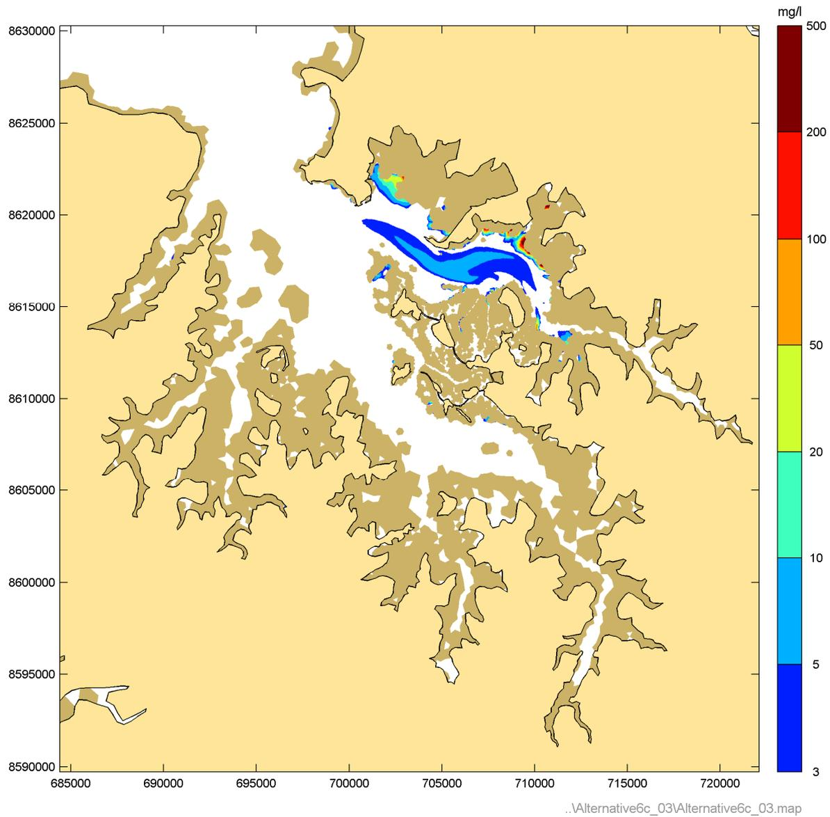
**Figure 50** Instantaneous suspended sediment concentrations during Phase 3 peak ebb – spring tide
