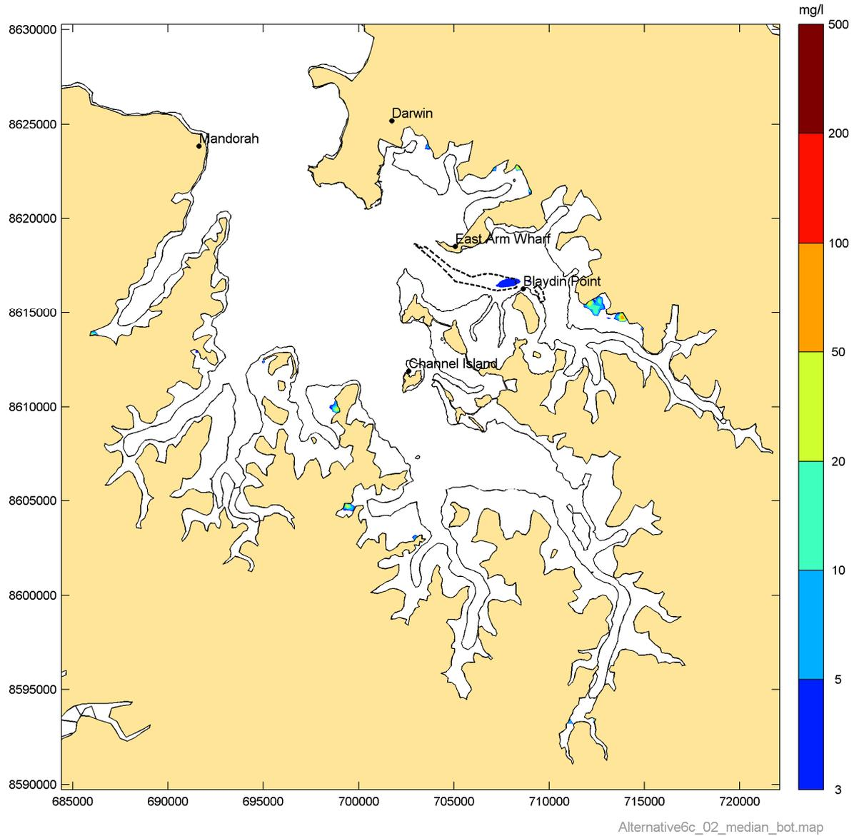
**Figure 19** Simulated median suspended sediment concentration in the East Arm for Phase 2
