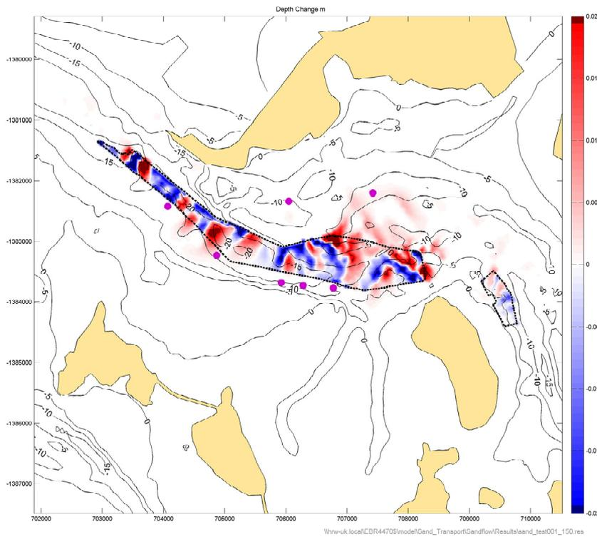
**Figure 136** Indicative areas of net erosion and deposition for spring-neap cycle 150 µm sand under tide-only conditions for predredge bathymetry (mobile material only within dredge footprint)
