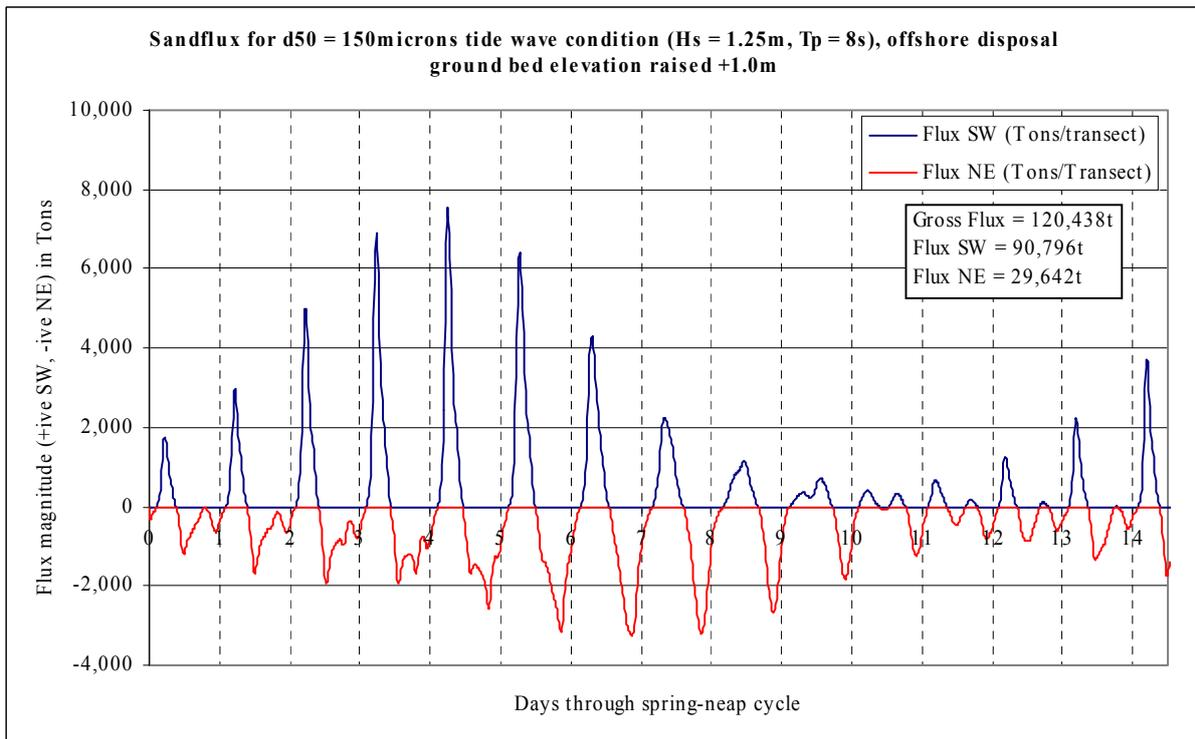
**Figure 148 Potential through tide sandflux magnitudes for spring-neap cycle for tide plus wave conditions and post-dredge bathymetry at the offshore disposal ground**
