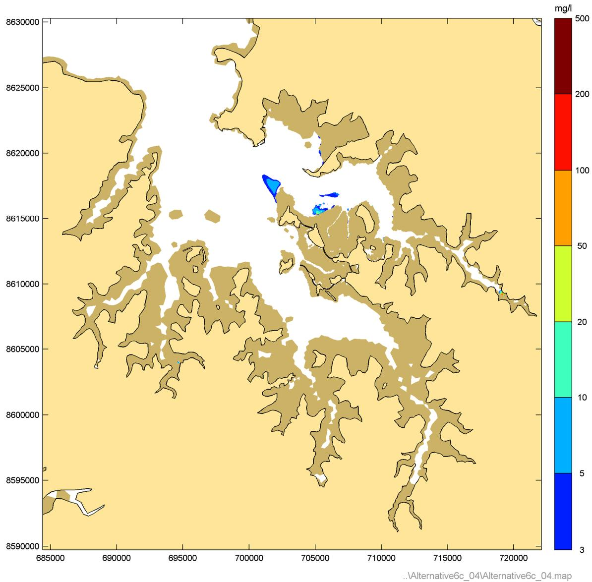
**Figure 52** Instantaneous suspended sediment concentrations during Phase 4 peak ebb – Neap tide
