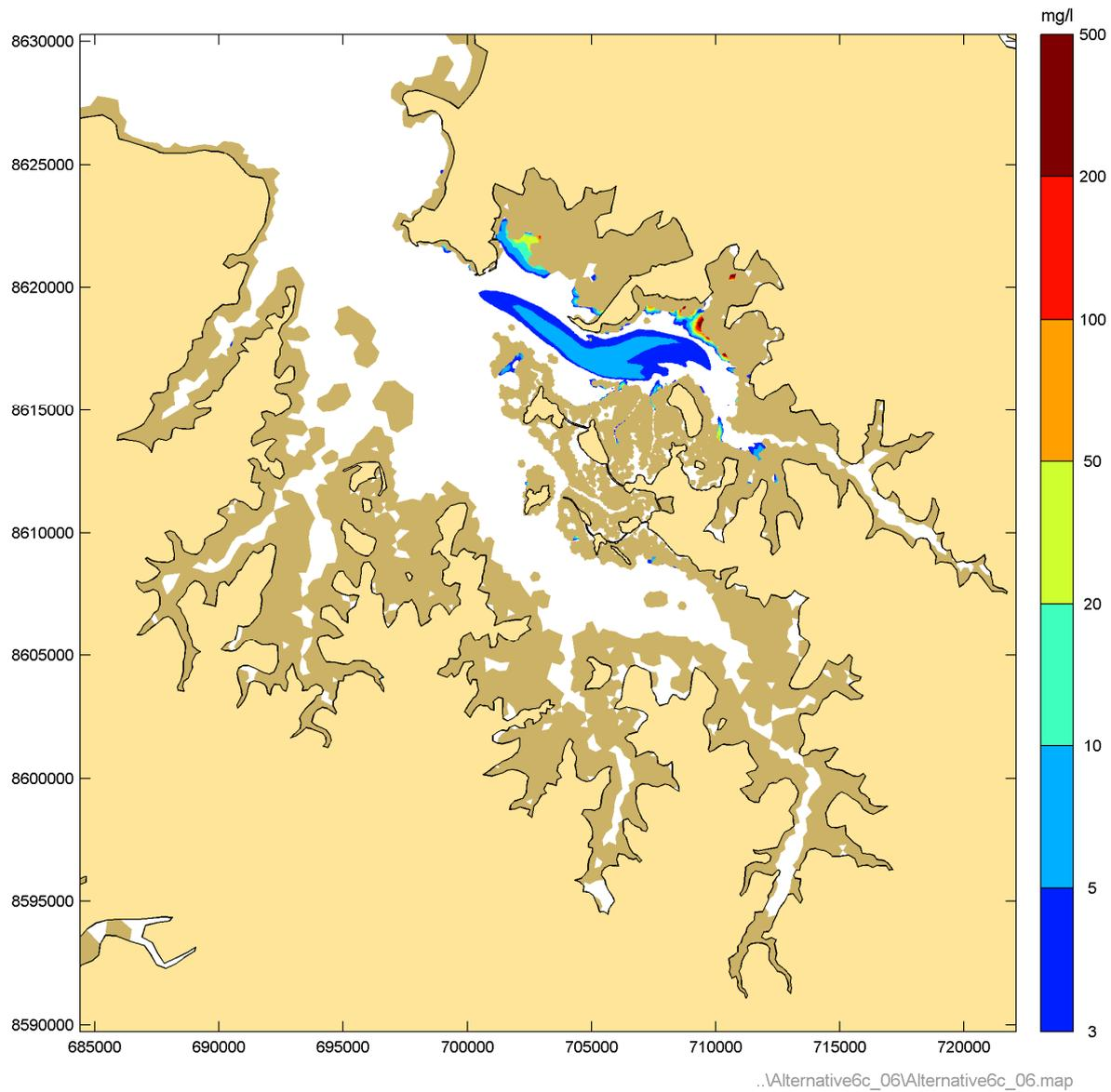
**Figure 64** Instantaneous suspended sediment concentrations during Phase 6 peak ebb – Spring tide
