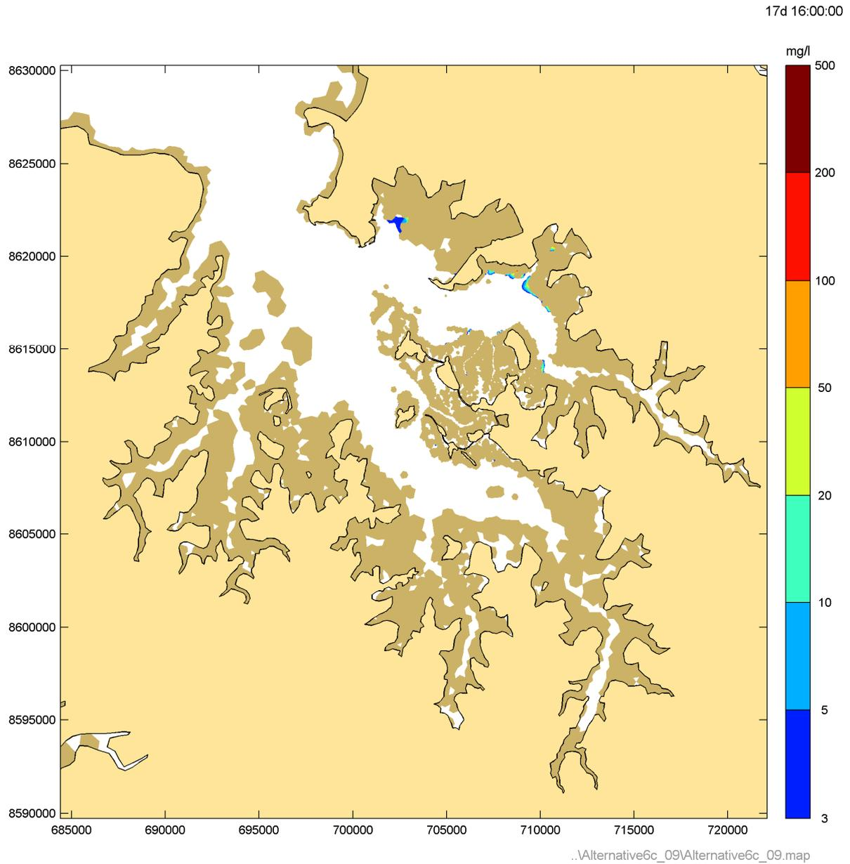
**Figure 78** Instantaneous suspended sediment concentrations during Phase 9 peak ebb – Spring tide
