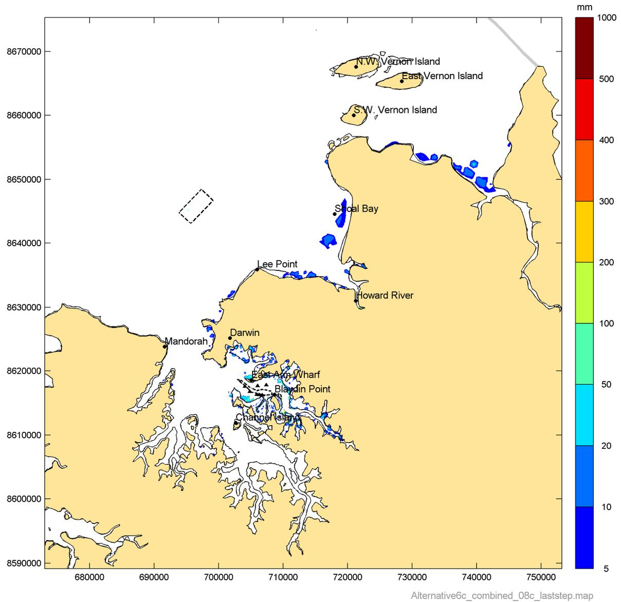
**Figure 123** Simulated depth of fine sediment accretion in the vicinity of Darwin Harbour at the end of Phase 8
