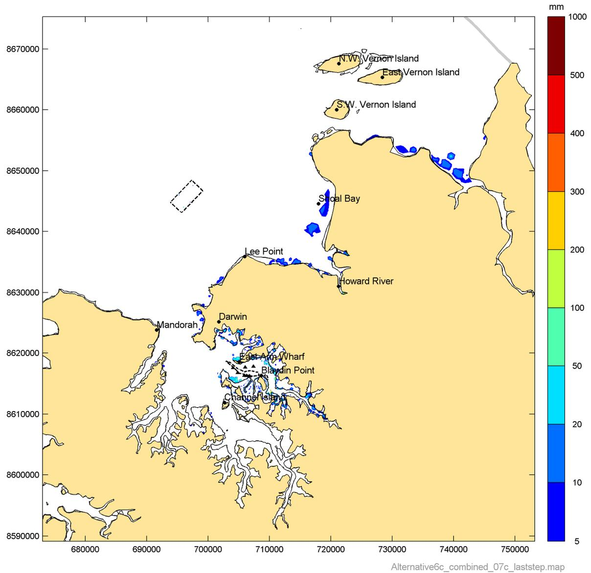
**Figure 122 Simulated depth of fine sediment accretion in the vicinity of Darwin Harbour at the end of Phase 7**
