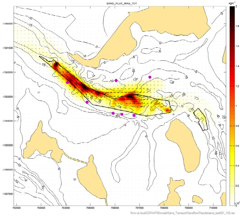
**Figure 135** Net sand transport for spring-neap cycle 150 µm sand under tide-only conditions for predredge bathymetry (mobile material only within dredge footprint)
