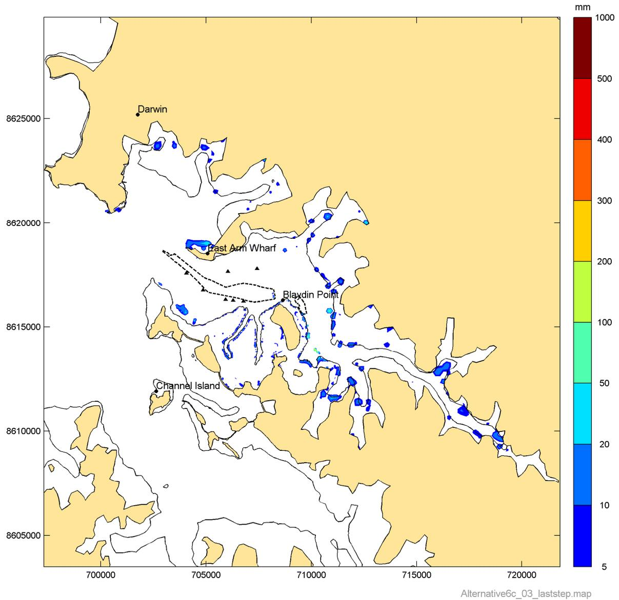
**Figure 86** Simulated depth of fine sediment accretion in the East Arm at the end of Phase 3
