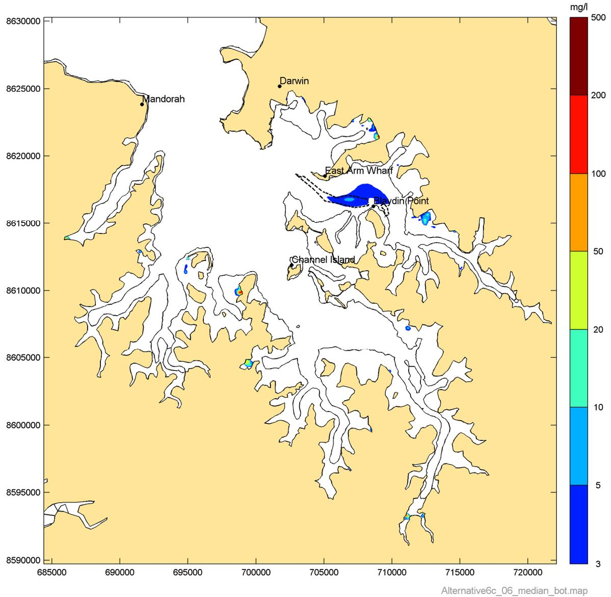
**Figure 23 Simulated median suspended sediment concentration in the East Arm for Phase 6**
