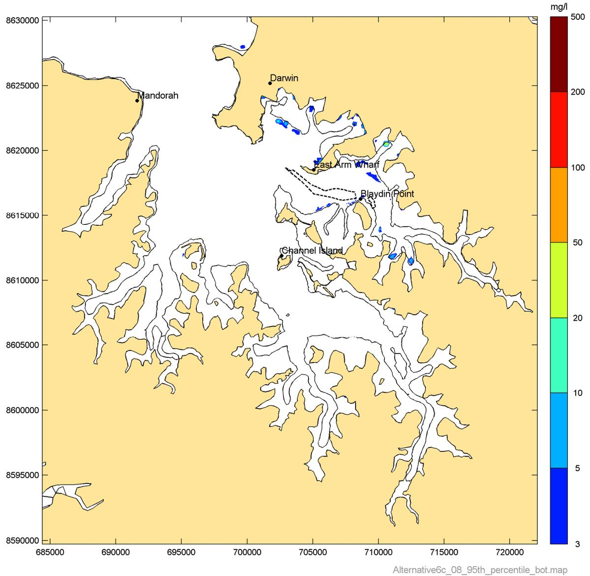
**Figure 37** Simulated 95<sup>th</sup> percentile suspended sediment concentration in the East Arm for Phase 8
