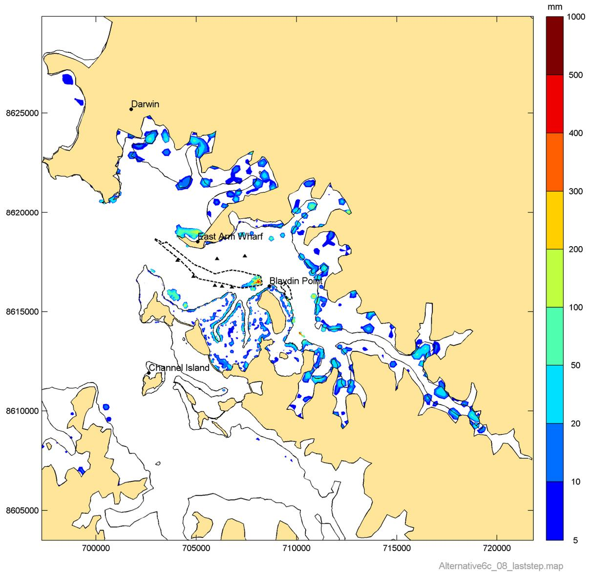
**Figure 91** Simulated depth of fine sediment accretion in the East Arm at the end of Phase 8
