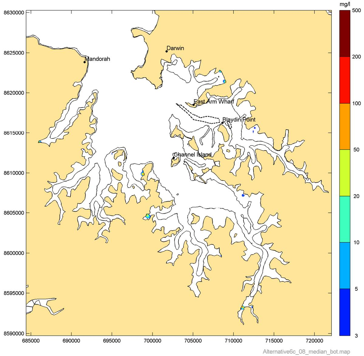
**Figure 26 Simulated median suspended sediment concentration in the East Arm for Phase 8**
