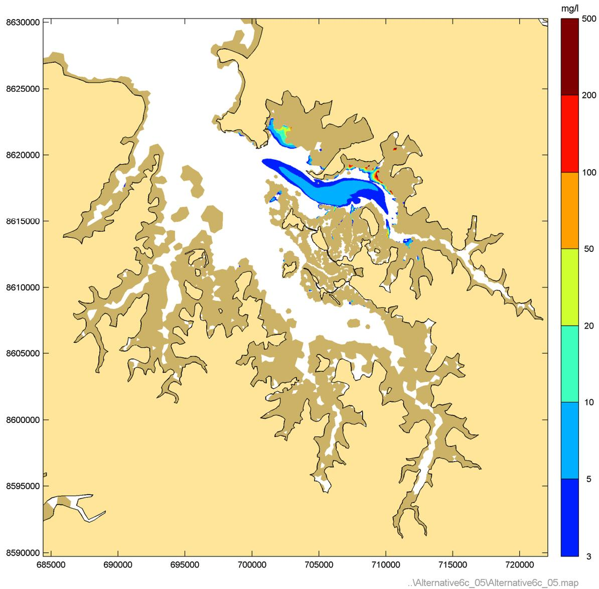
**Figure 58** Instantaneous suspended sediment concentrations during Phase 5 peak ebb – Spring tide
