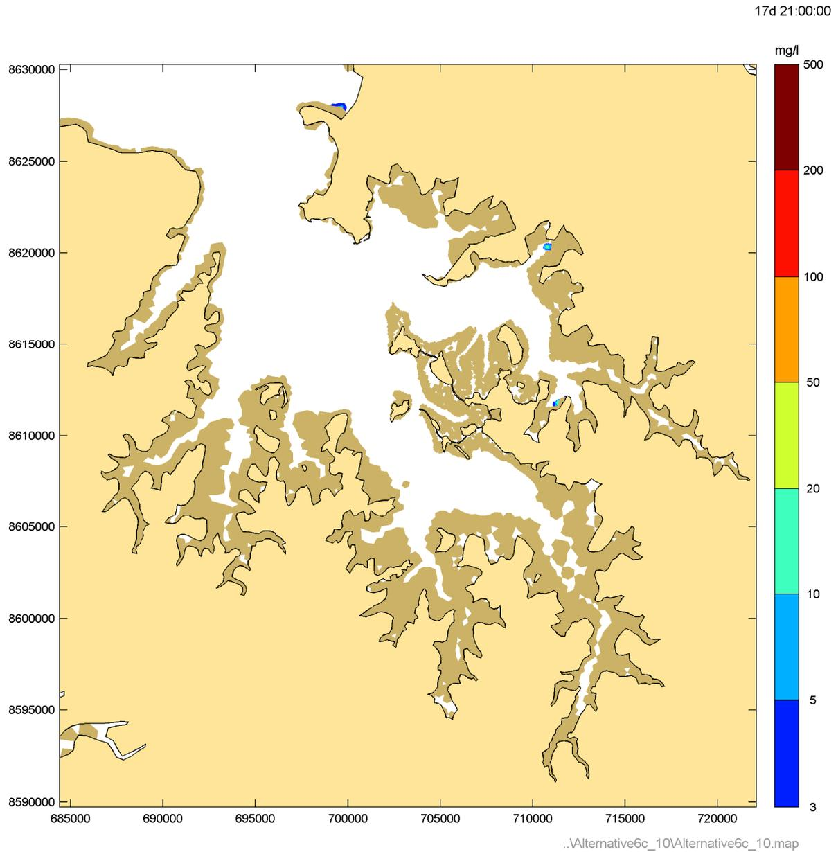
**Figure 83** Instantaneous suspended sediment concentrations during Phase 10 peak flood – Spring tide
