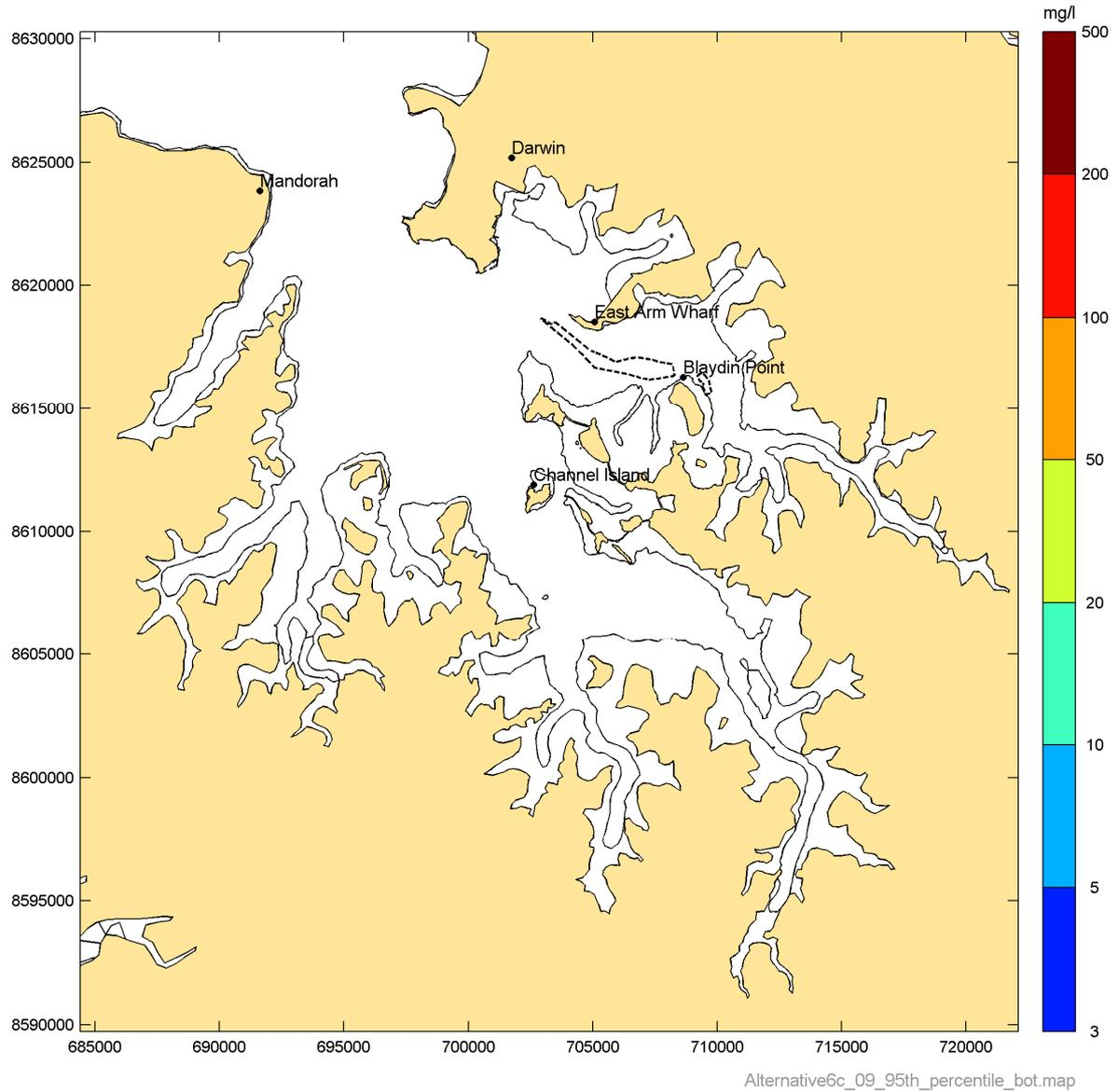
**Figure 38** Simulated 95<sup>th</sup> percentile suspended sediment concentration in the East Arm for Phase 9
