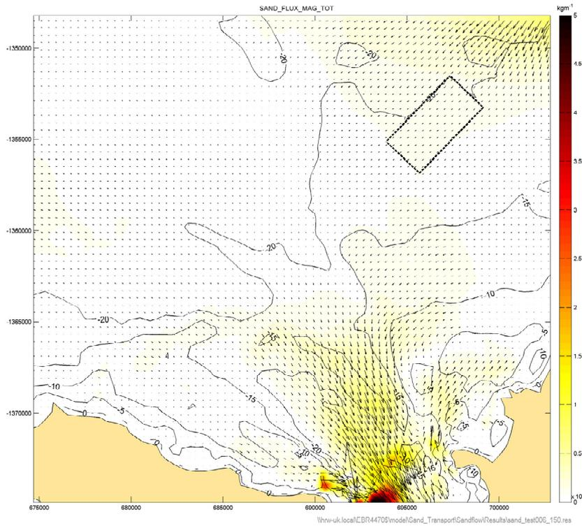
**Figure 143 Net sand transport for spring-neap cycle 150 µm sand under tide-only conditions for post-dredge bathymetry (offshore disposal ground +1.0m)**
