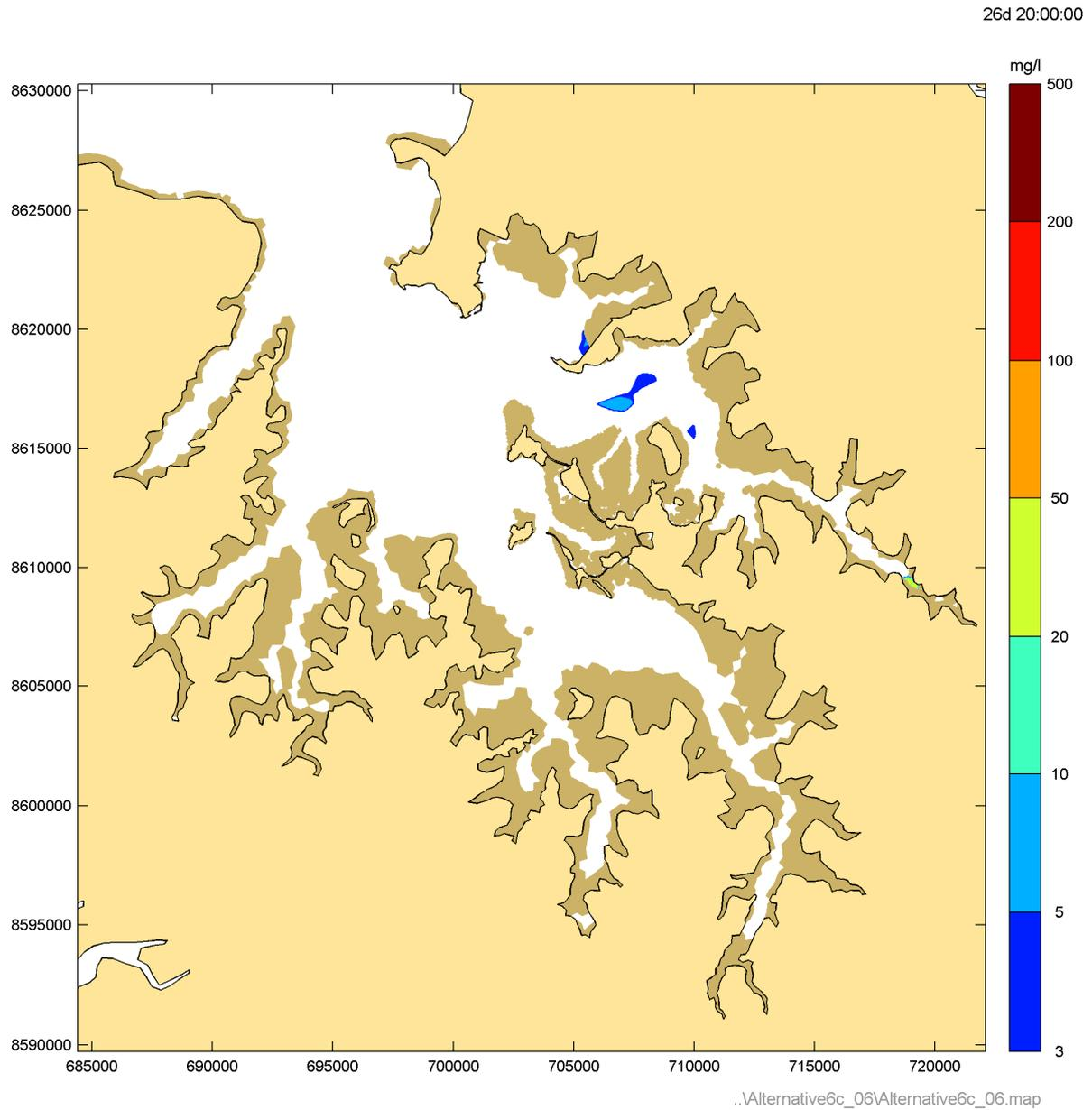
**Figure 62** Instantaneous suspended sediment concentrations during Phase 6 peak flood – Neap tide
