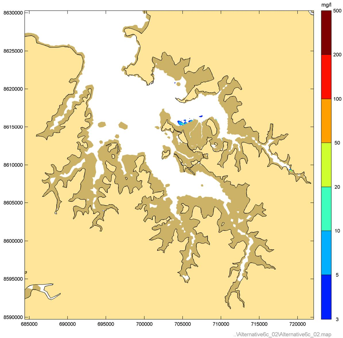
**Figure 44** Instantaneous suspended sediment concentrations during Phase 2 peak ebb – Neap tide
