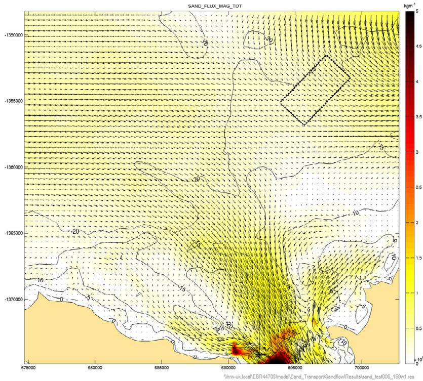
**Figure 145** Net sand transport for spring-neap cycle 150 µm sand under tide plus wave conditions for post-dredge bathymetry (offshore disposal ground +1.0m)
