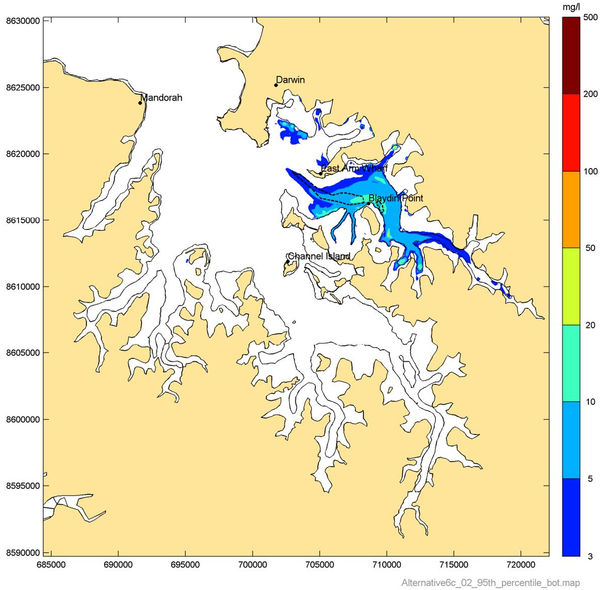
**Figure 30** Simulated 95<sup>th</sup> percentile suspended sediment concentration in the East Arm for Phase 2
