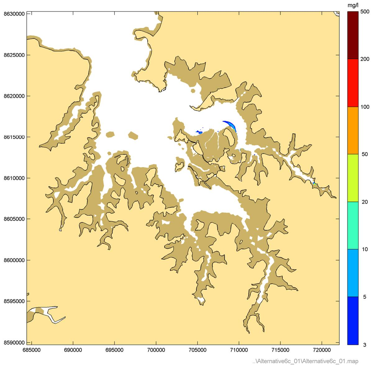
**Figure 40** Instantaneous suspended sediment concentrations during Phase 1 peak ebb – Neap tide
