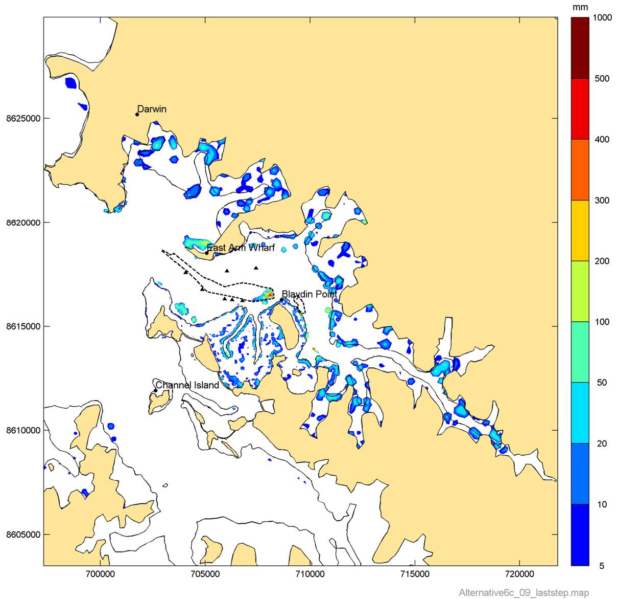
**Figure 92** Simulated depth of fine sediment accretion in the East Arm at the end of Phase 9
