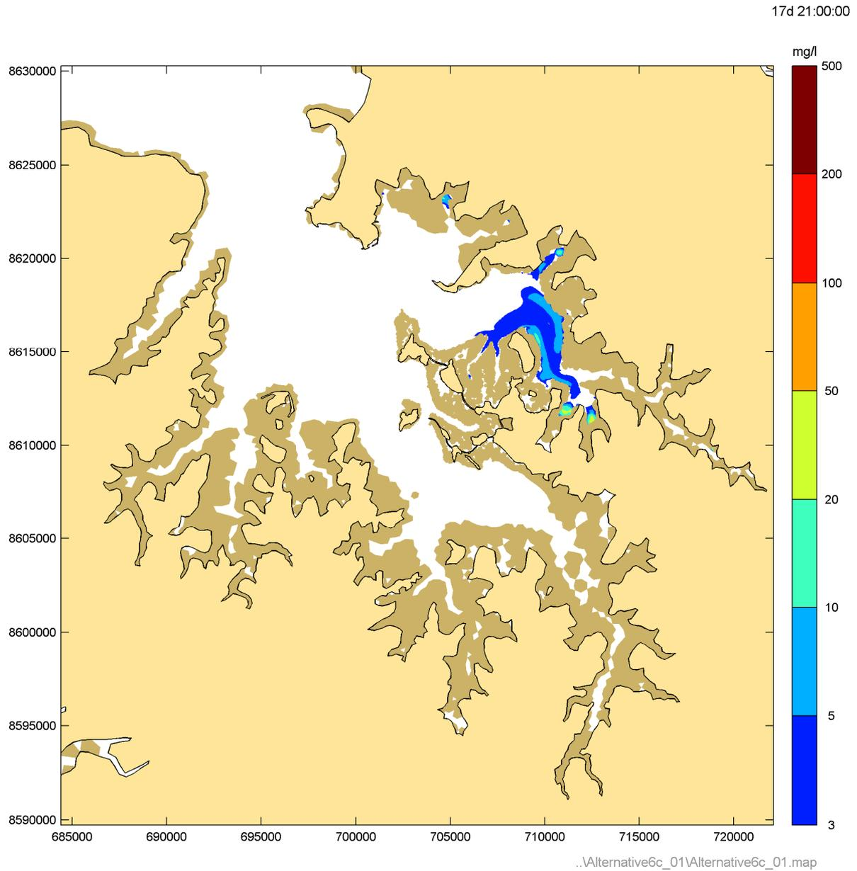
**Figure 43** Instantaneous suspended sediment concentrations during Phase 1 peak flood – spring tide
