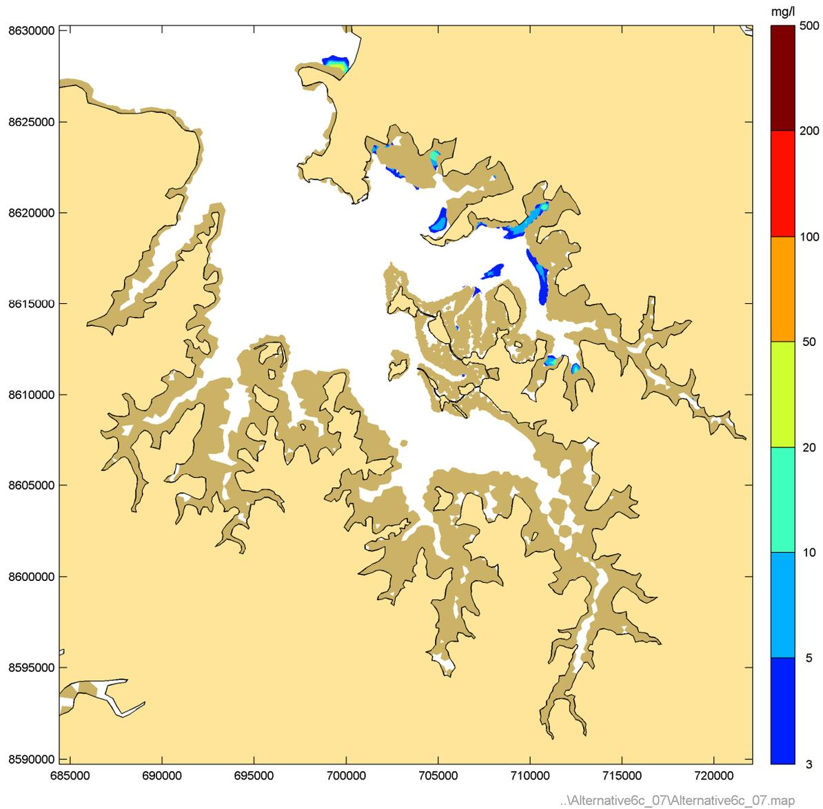
**Figure 71** Instantaneous suspended sediment concentrations during Phase 7 peak flood – Spring tide
