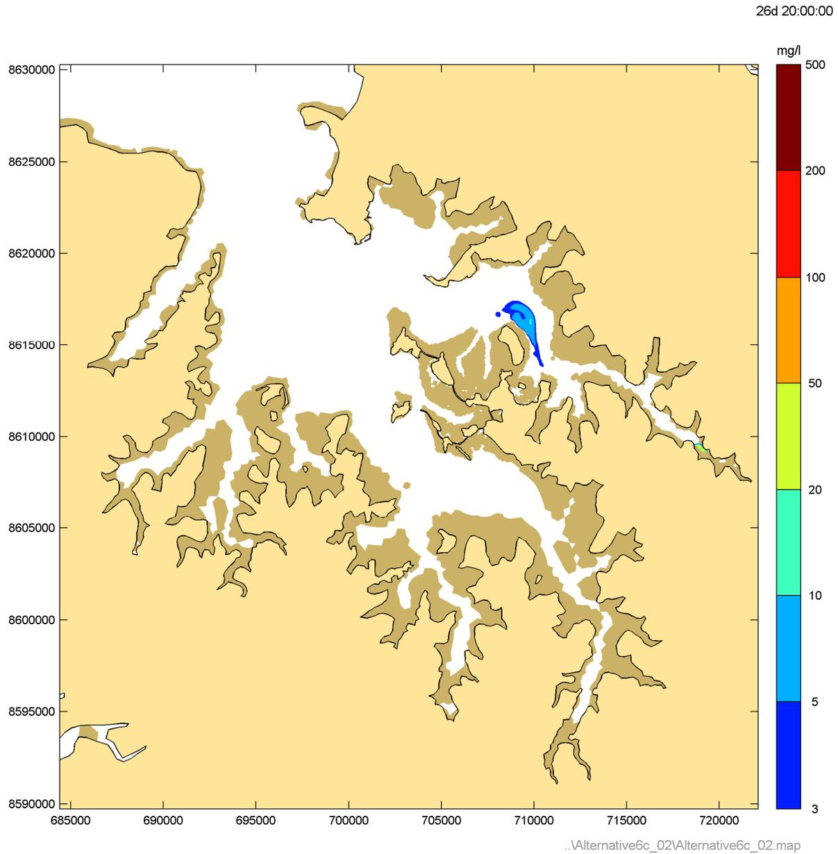
**Figure 45** Instantaneous suspended sediment concentrations during Phase 2 peak flood – Neap tide
