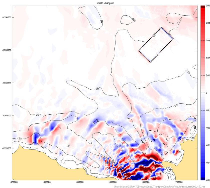
**Figure 144 Indicative areas of net erosion and deposition for spring-neap cycle 150 µm sand under tide-only conditions for post-dredge bathymetry (offshore disposal ground +1.0m)**
