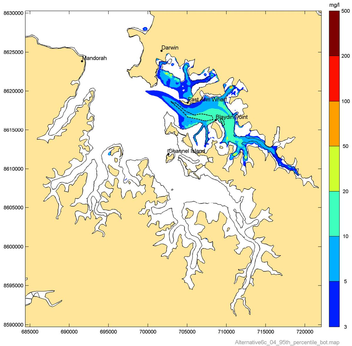
**Figure 32** Simulated 95<sup>th</sup> percentile suspended sediment concentration in the East Arm for Phase 4
