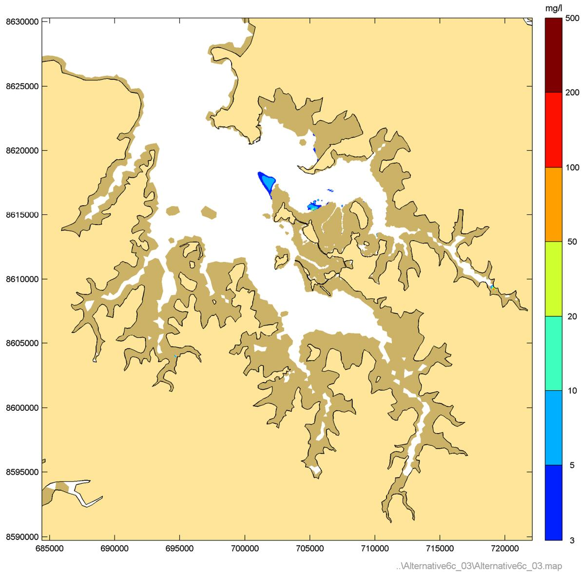
**Figure 48** Instantaneous suspended sediment concentrations during Phase 3 peak ebb – Neap tide
