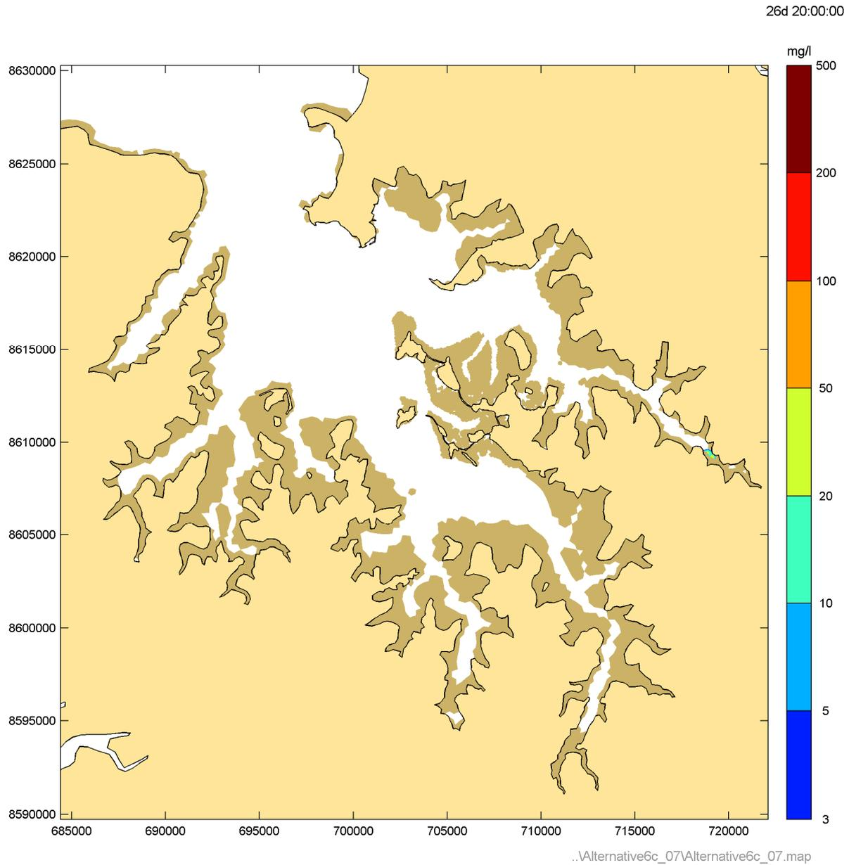
**Figure 69** Instantaneous suspended sediment concentrations during Phase 7 peak flood – Neap tide
