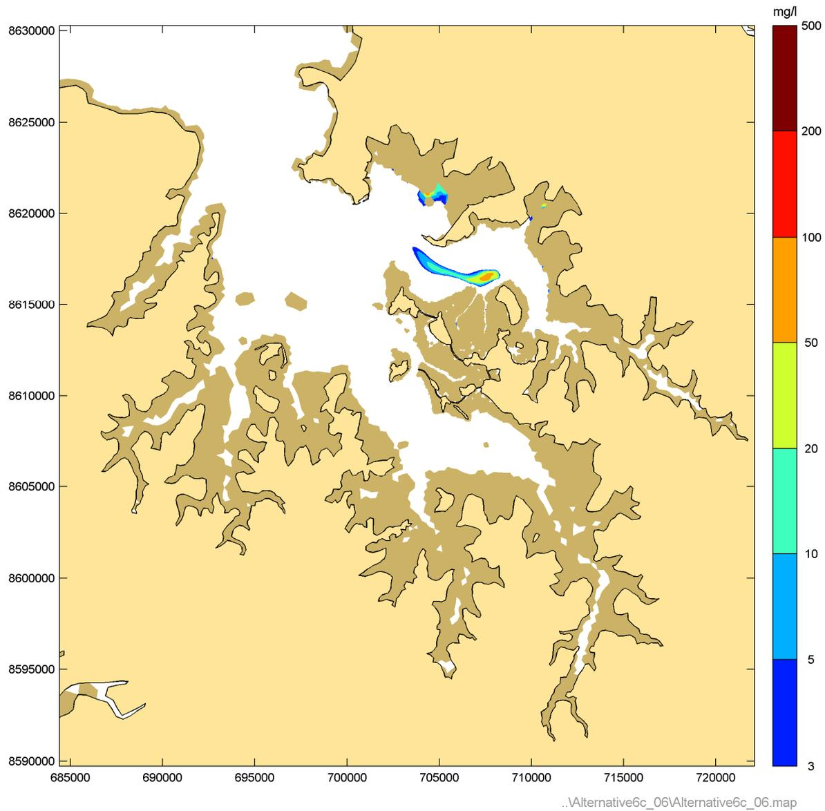
**Figure 61** Instantaneous suspended sediment concentrations during Phase 6 peak ebb – Neap tide (cutter-suction dredger activity)
