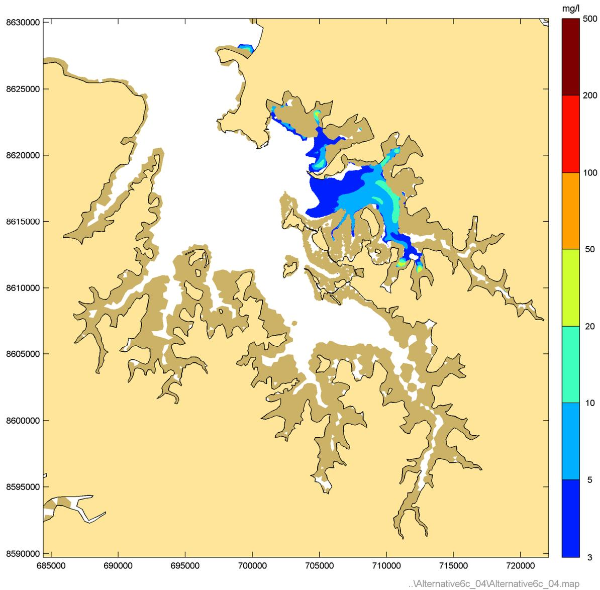
**Figure 55** Instantaneous suspended sediment concentrations during Phase 4 peak flood – Spring tide
