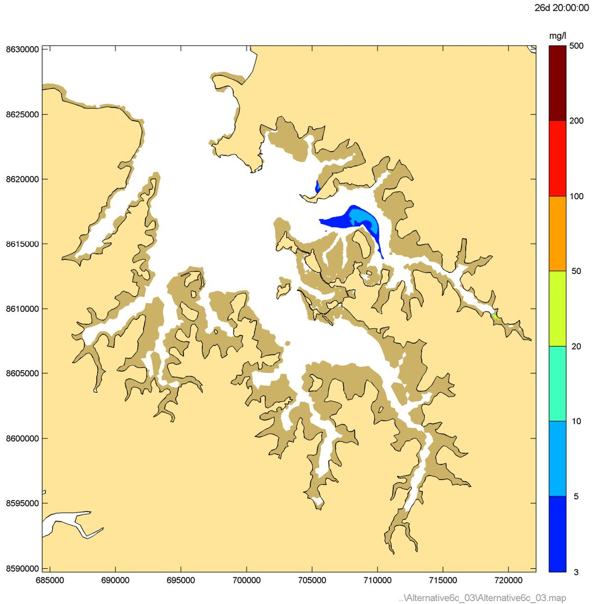
**Figure 49** Instantaneous suspended sediment concentrations during Phase 3 peak flood – Neap tide
