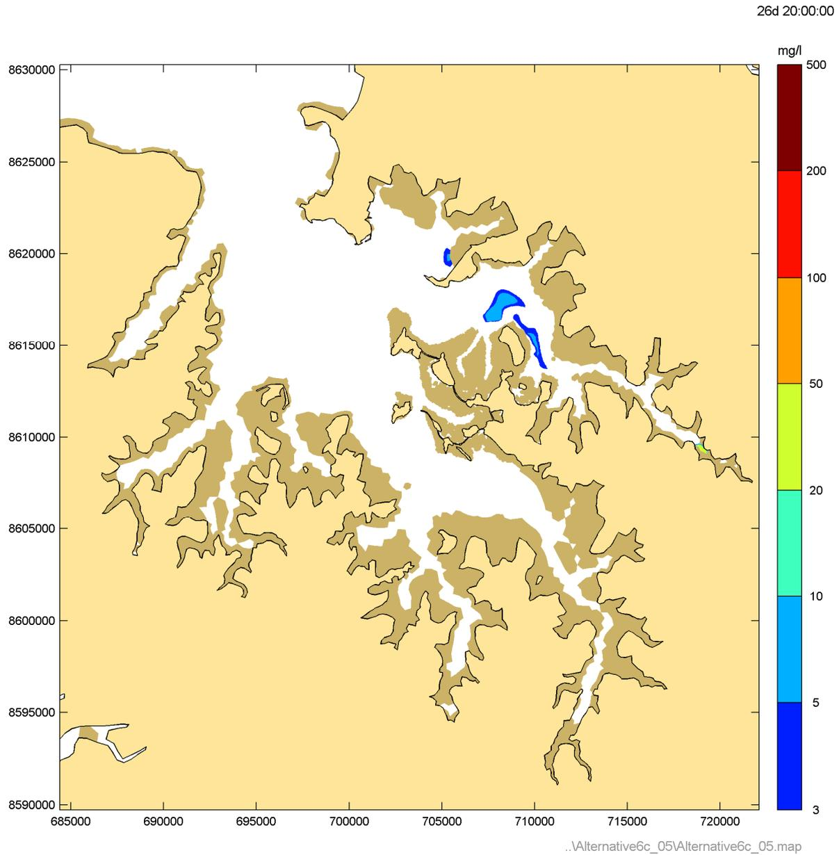
**Figure 57** Instantaneous suspended sediment concentrations during Phase 5 peak flood – Neap tide
