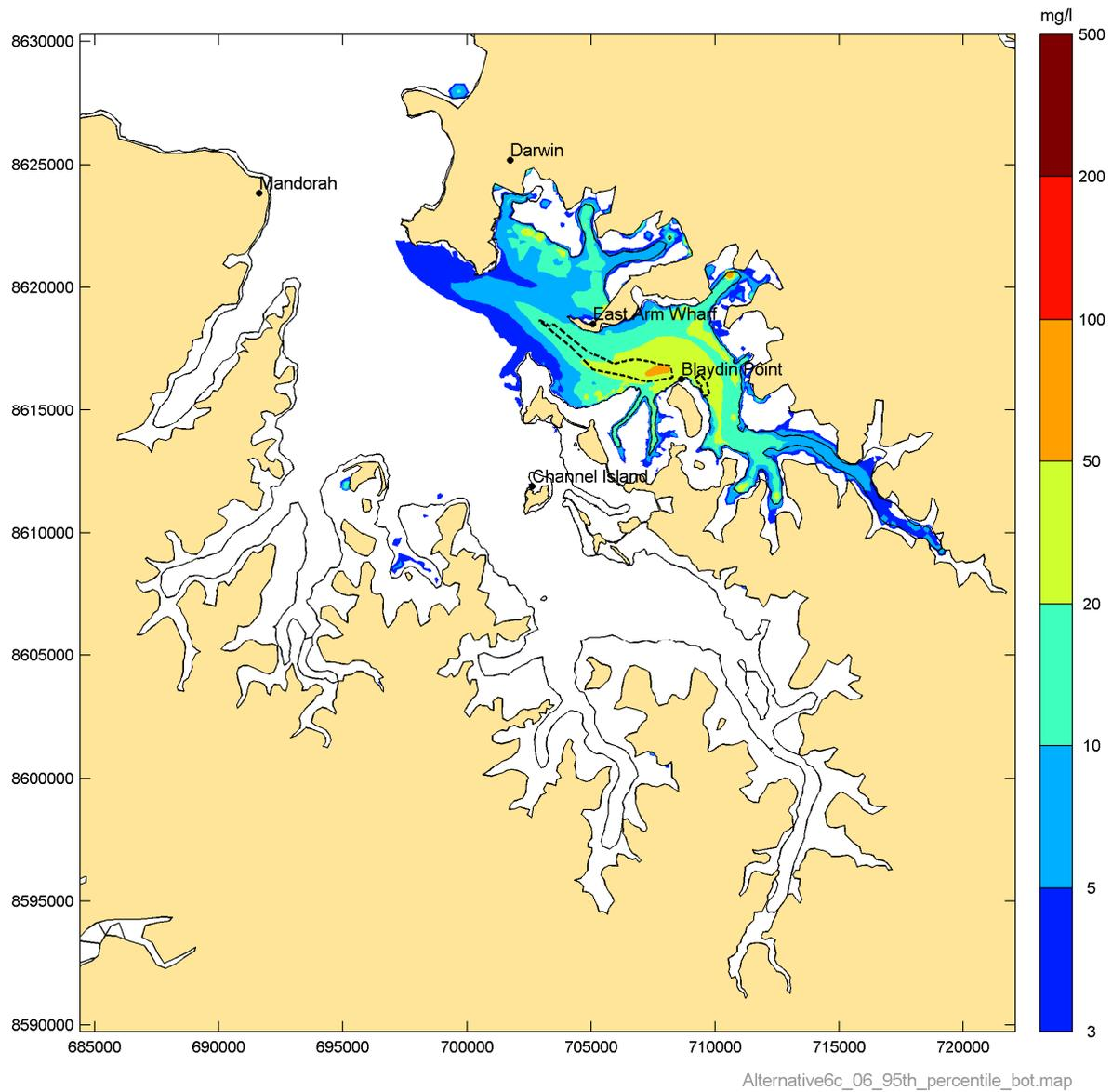
**Figure 34** Simulated 95<sup>th</sup> percentile suspended sediment concentration in the East Arm for Phase 6
