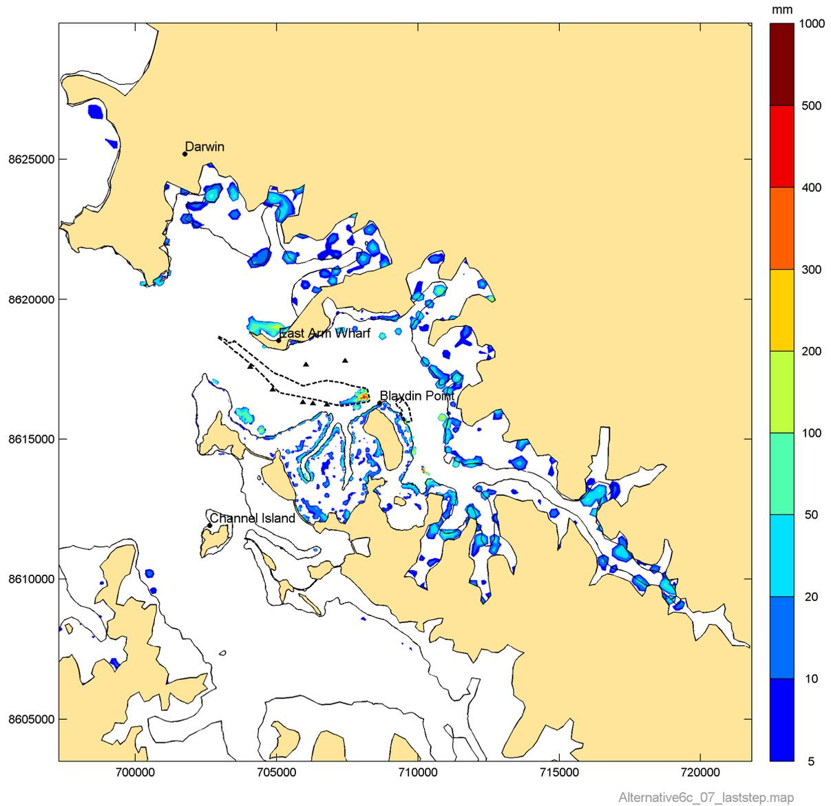
**Figure 90** Simulated depth of fine sediment accretion in the East Arm at the end of Phase 7
