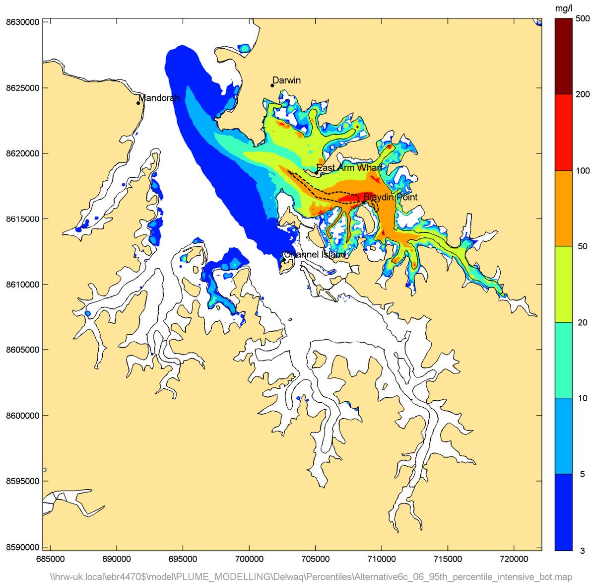
**Figure 35** Simulated 95<sup>th</sup> percentile suspended sediment concentration in the East Arm for Phase 6 – cutter-suction dredger activity
