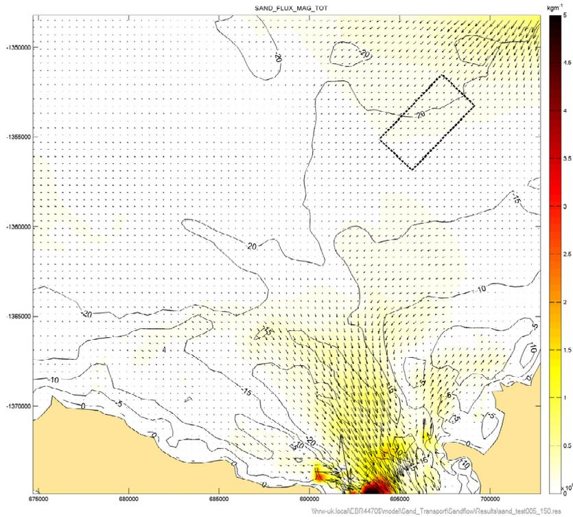
**Figure 137** Net sand transport for spring-neap cycle 150 µm sand under tide-only conditions for pre-dredge bathymetry
