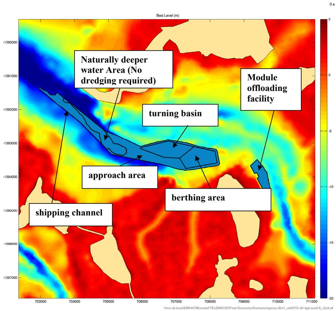
**Figure 3** Defined areas used to simulate fine material release in the sediment transport model within the East Arm
