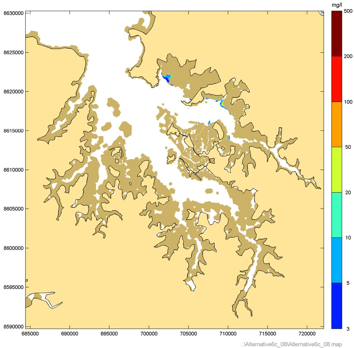
**Figure 74** Instantaneous suspended sediment concentrations during Phase 8 peak ebb – Spring tide
