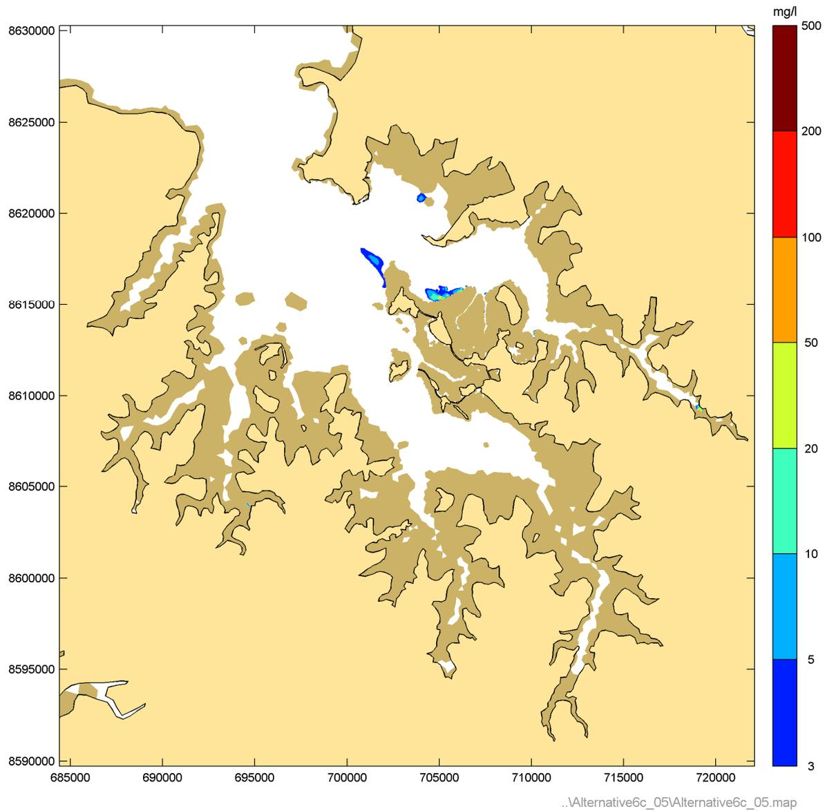
**Figure 56** Instantaneous suspended sediment concentrations during Phase 5 peak ebb – Neap tide
