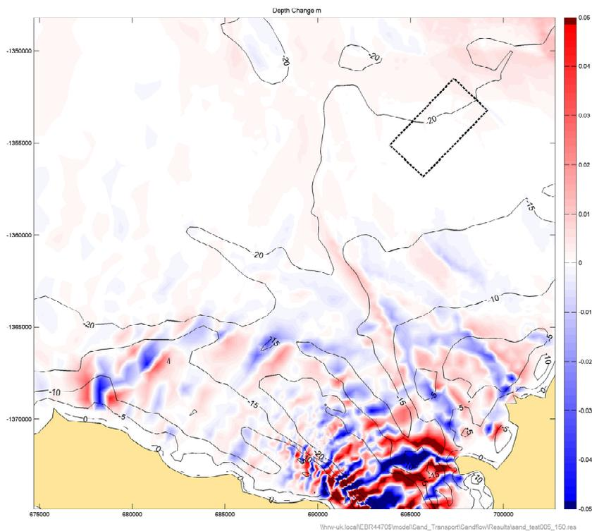
**Figure 138** Indicative areas of net erosion and deposition for spring-neap cycle 150 µm sand under tide-only conditions for pre-dredge bathymetry.
