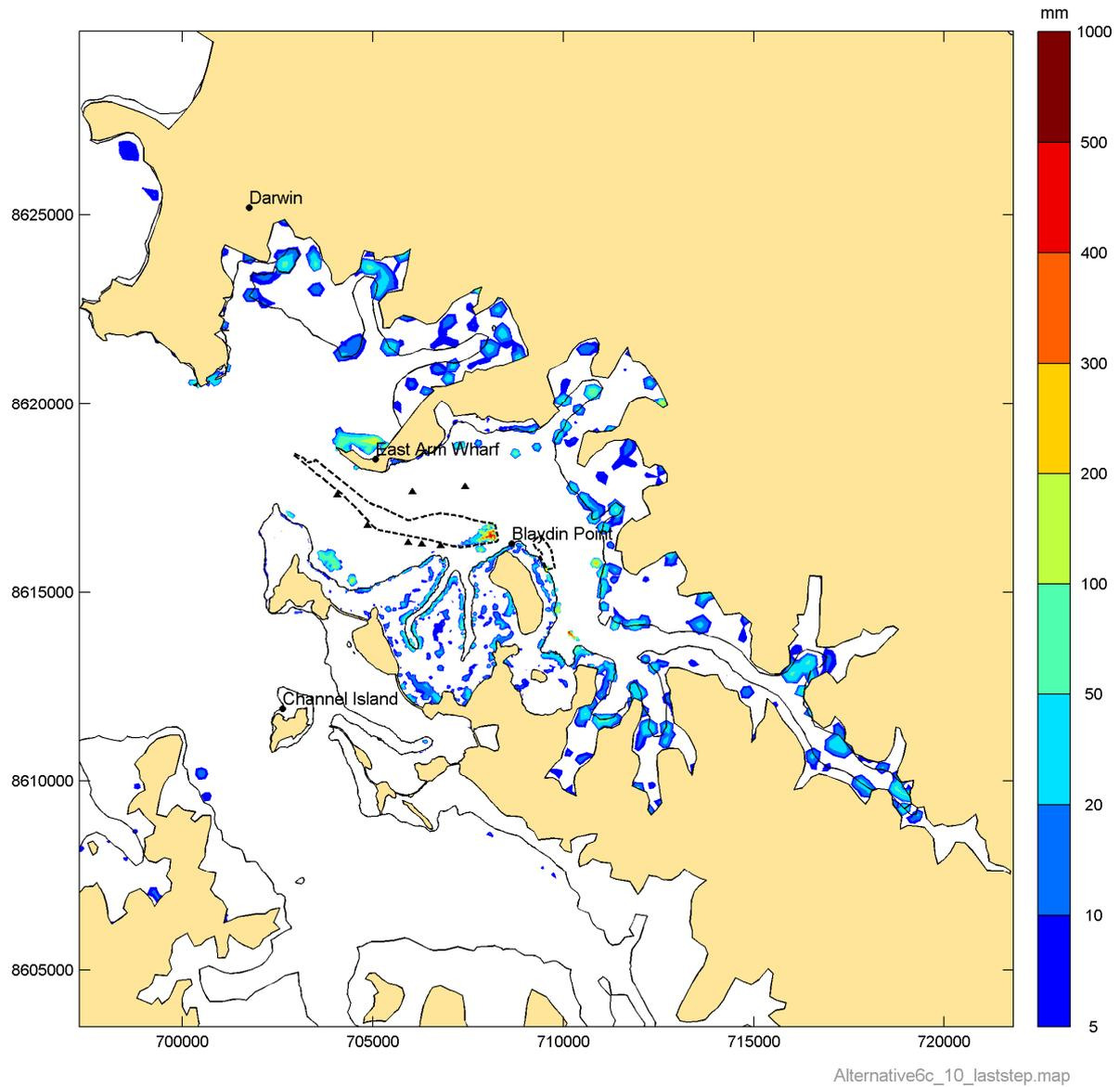
**Figure 93** Simulated depth of fine sediment accretion in the East Arm at the end of Phase 10
