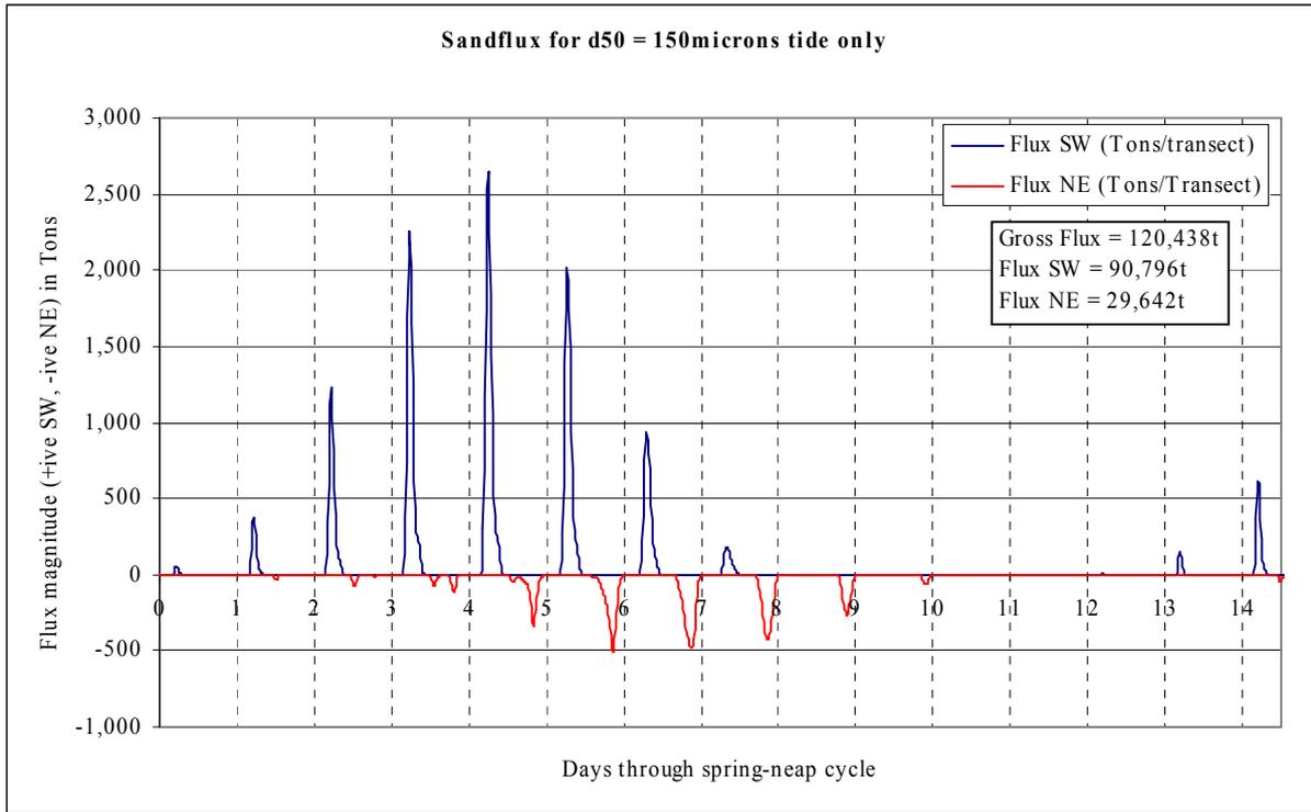
**Figure 141** Potential through tide sandflux magnitudes for spring-neap cycle for tide-only conditions and pre-dredge bathymetry at the offshore disposal ground
