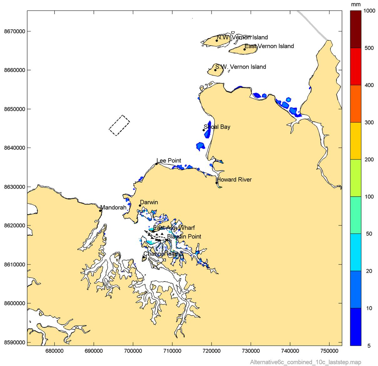
**Figure 125 Simulated depth of fine sediment accretion in the vicinity of Darwin Harbour at the end of Phase 10**
