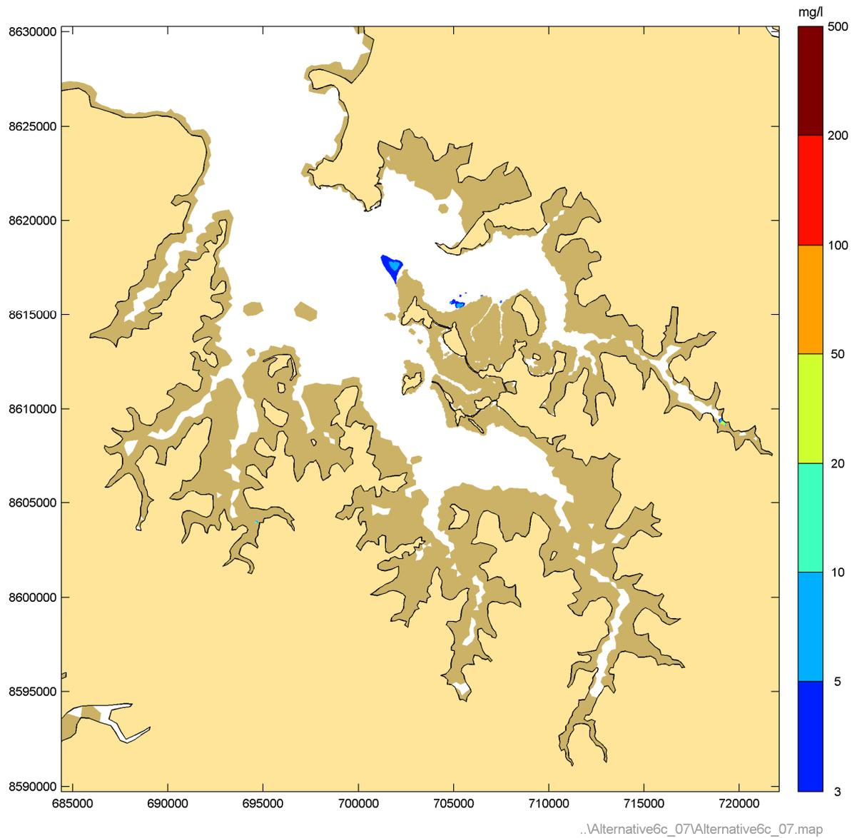
**Figure 68** Instantaneous suspended sediment concentrations during Phase 7 peak ebb – Neap tide
