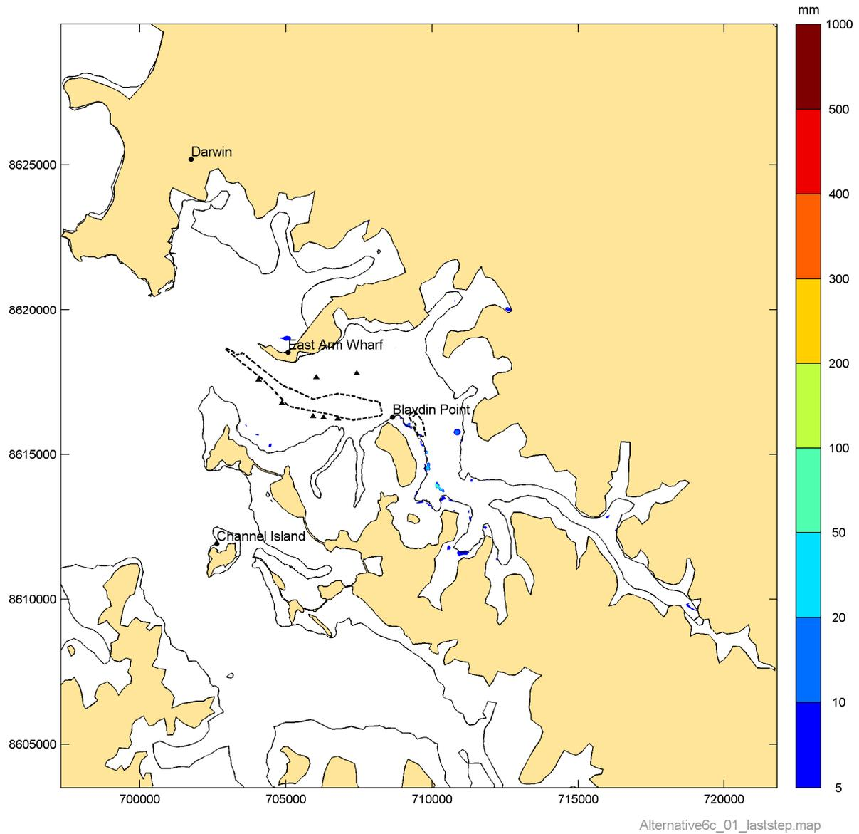
**Figure 84** Simulated depth of fine sediment accretion in the East Arm at the end of Phase 1
