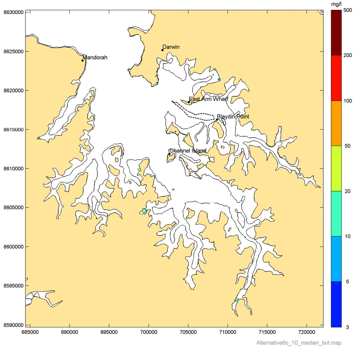
**Figure 28 Simulated median suspended sediment concentration in the East Arm for Phase 10**
