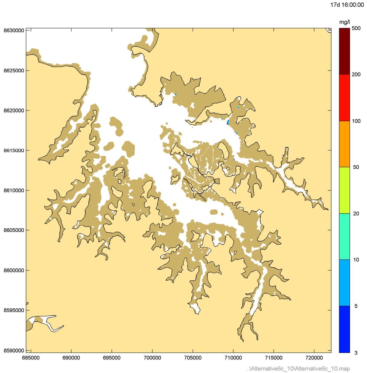
**Figure 82** Instantaneous suspended sediment concentrations during Phase 10 peak ebb – Spring tide
