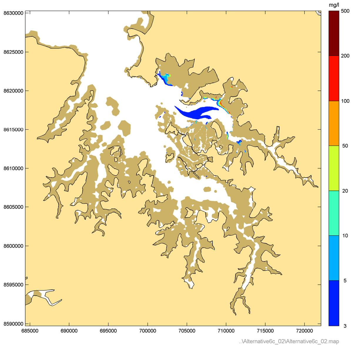
**Figure 46** Instantaneous suspended sediment concentrations during Phase 2 peak ebb – spring tide
