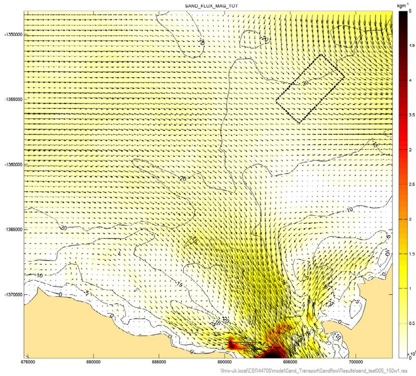
**Figure 139** Net sand transport for spring-neap cycle 150 µm sand under tide plus wave conditions for pre-dredge bathymetry
