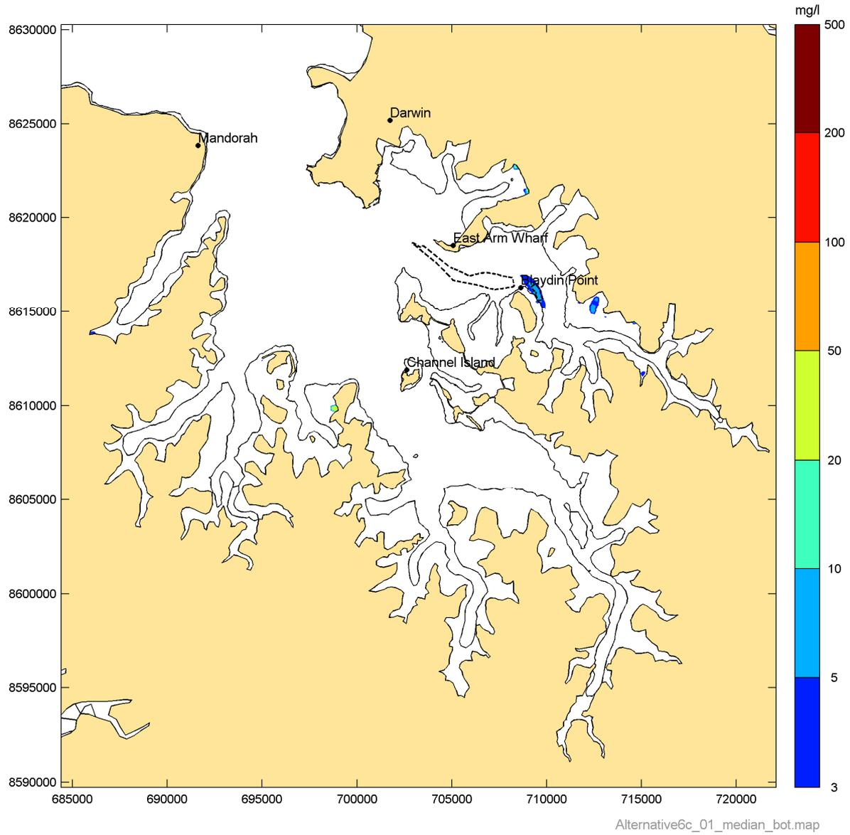
**Figure 18 Simulated median suspended sediment concentration in the East Arm for Phase 1**
