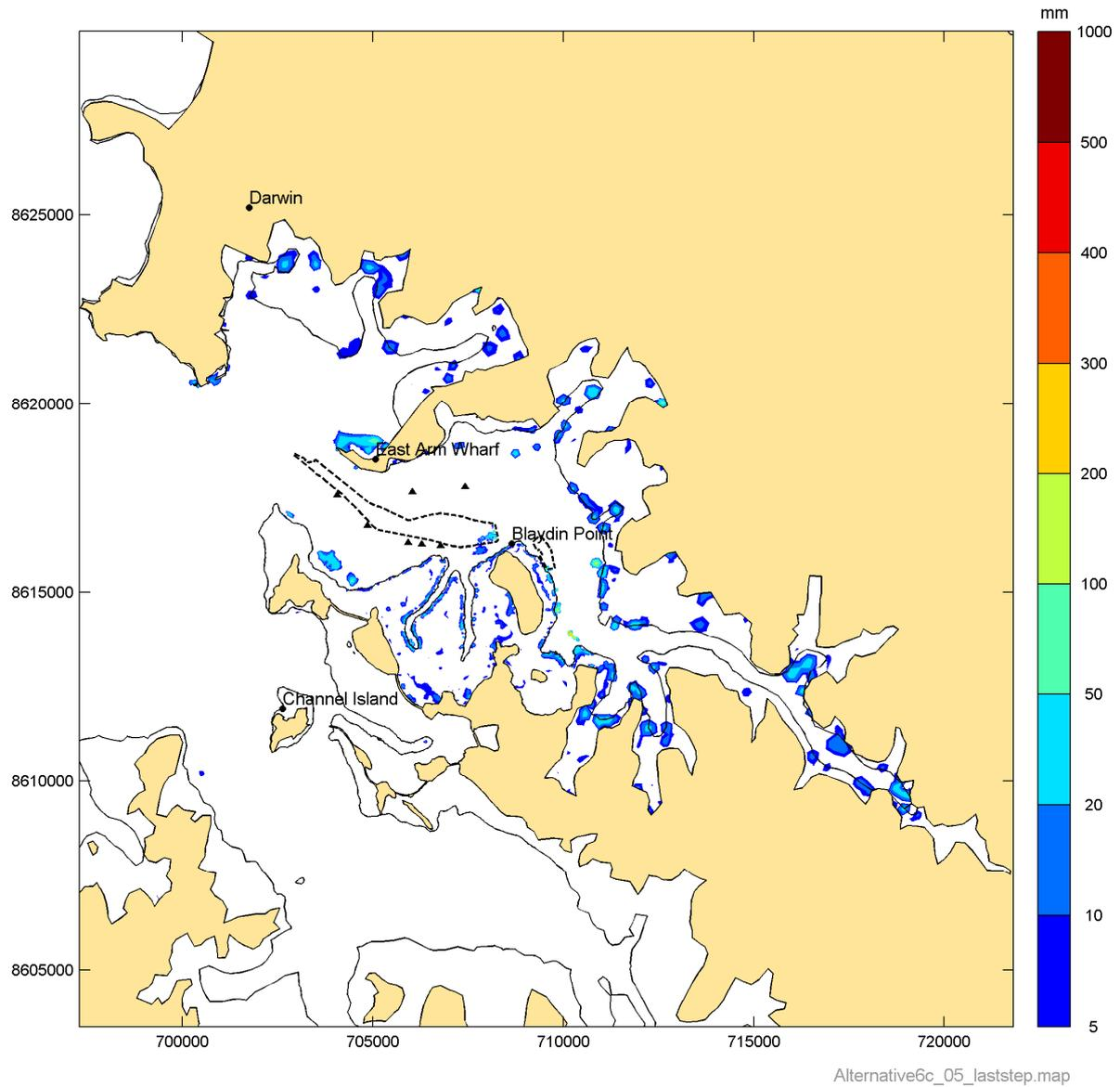
**Figure 88** Simulated depth of fine sediment accretion in the East Arm at the end of Phase 5
