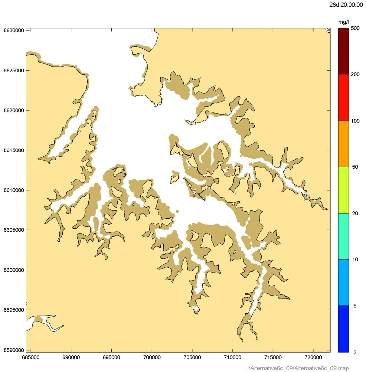
**Figure 77** Instantaneous suspended sediment concentrations during Phase 9 peak flood – Neap tide
