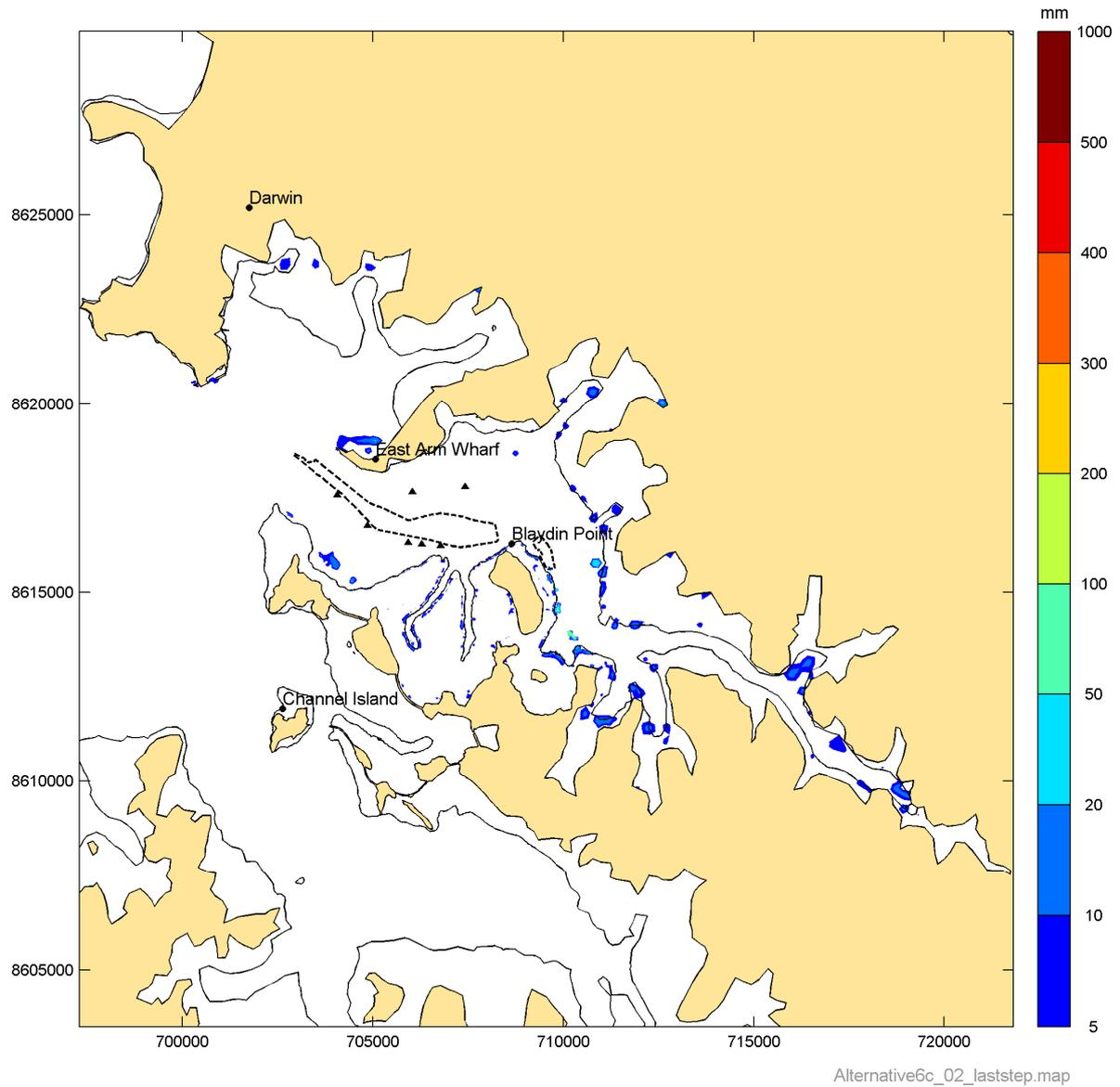
**Figure 85** Simulated depth of fine sediment accretion in the East Arm at the end of Phase 2
