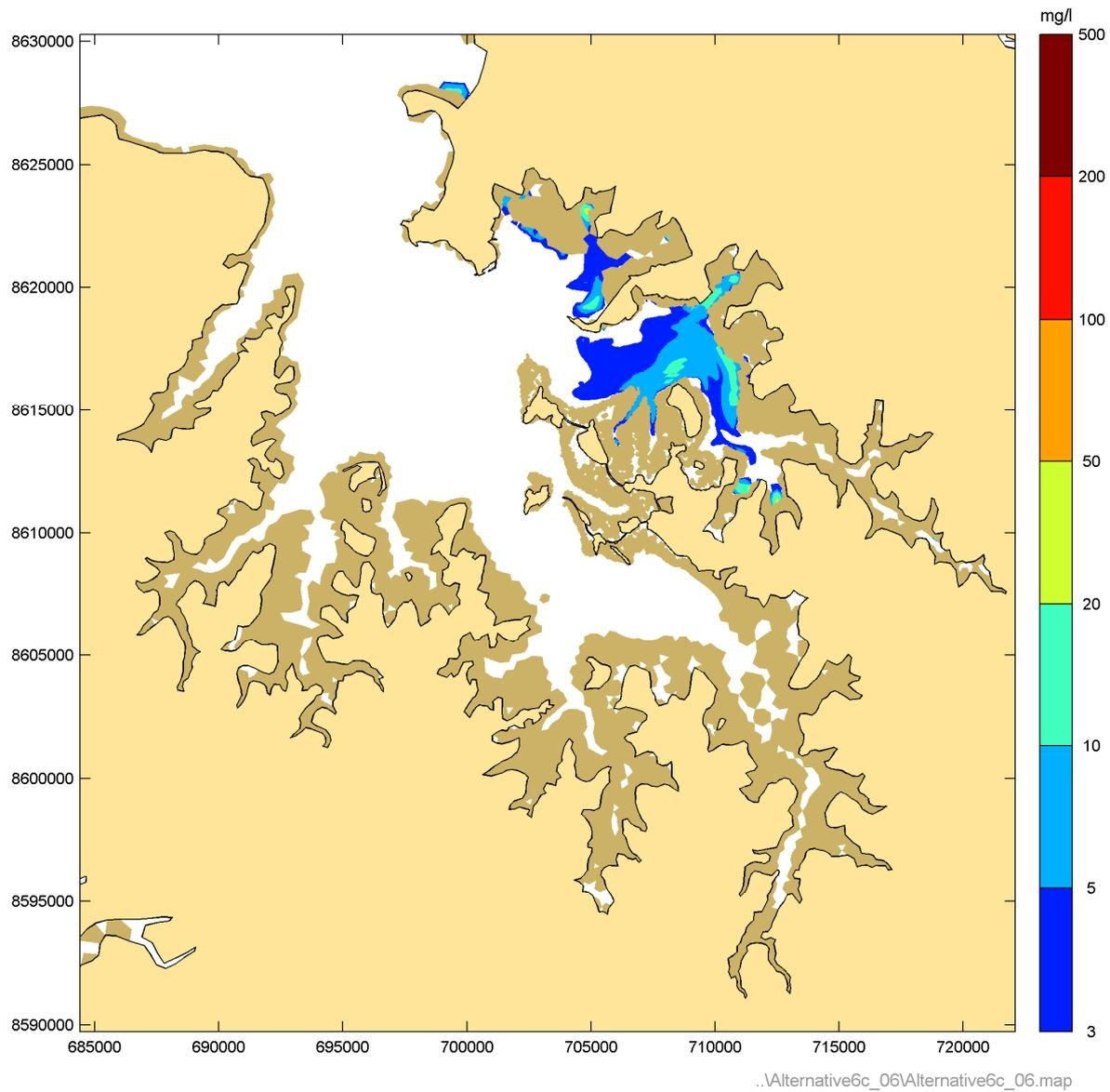
**Figure 66** Instantaneous suspended sediment concentrations during Phase 6 peak flood – Spring tide
