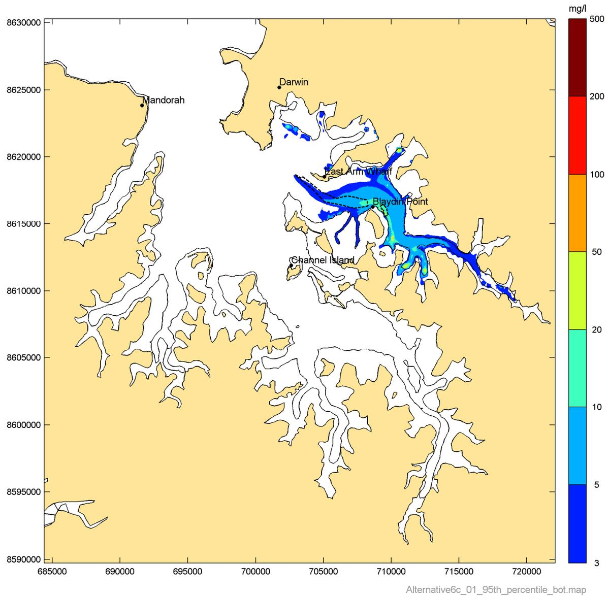
**Figure 29** Simulated 95<sup>th</sup> percentile suspended sediment concentration in the East Arm for Phase 1
