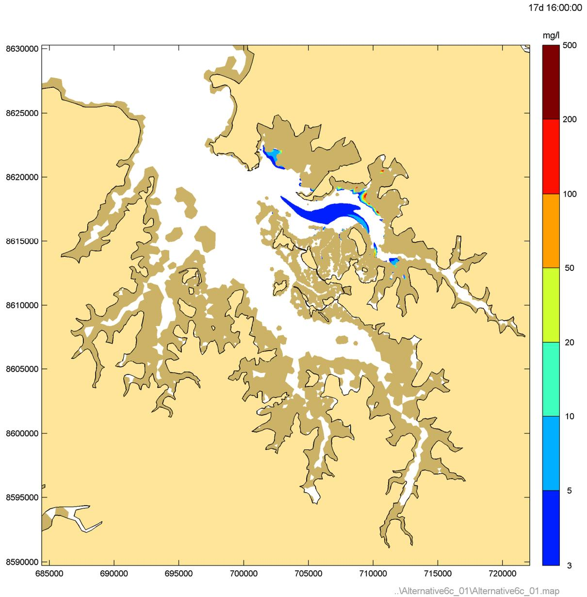
**Figure 42** Instantaneous suspended sediment concentrations during Phase 1 peak ebb – spring tide
