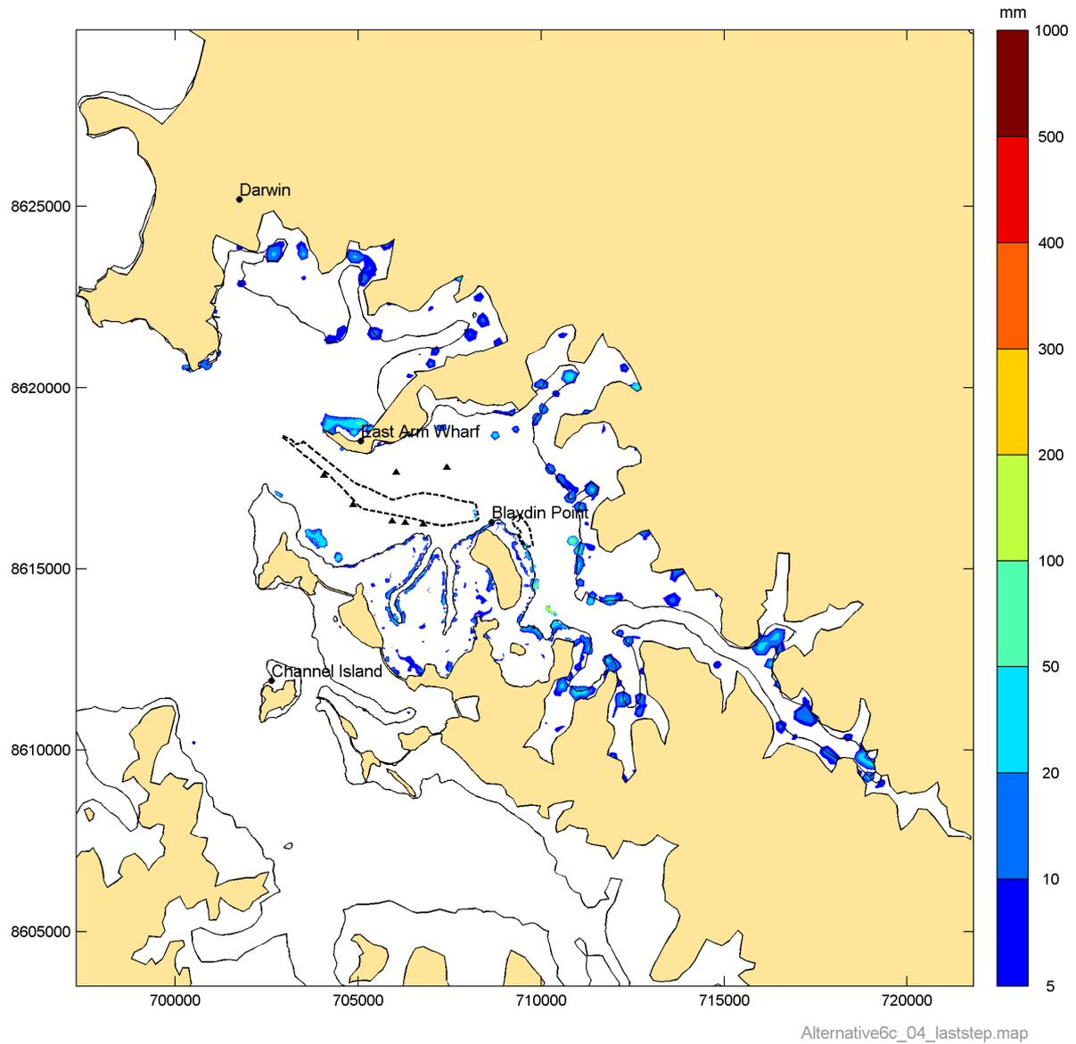
**Figure 87** Simulated depth of fine sediment accretion in the East Arm at the end of Phase 4
