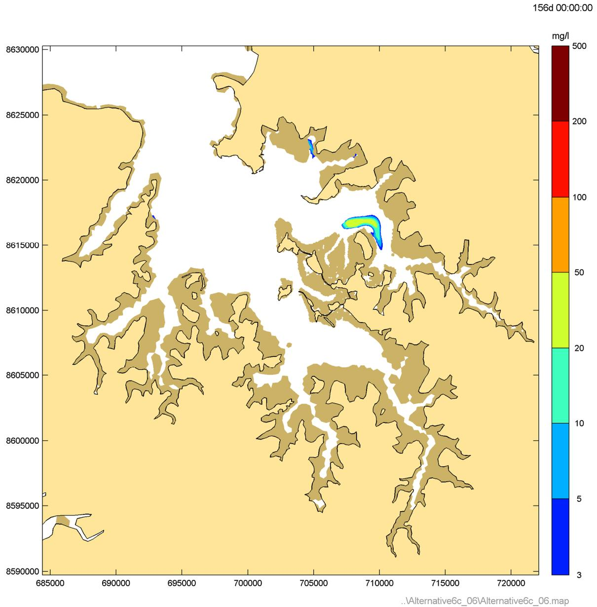
**Figure 63** Instantaneous suspended sediment concentrations during Phase 6 peak flood – Neap tide (cutter-suction dredger activity)
