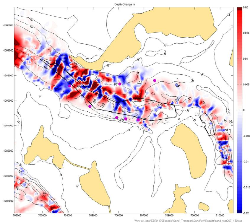
**Figure 131** Indicative areas of net erosion and deposition for spring-neap cycle 150 µm sand under tide-only conditions for predredge bathymetry
