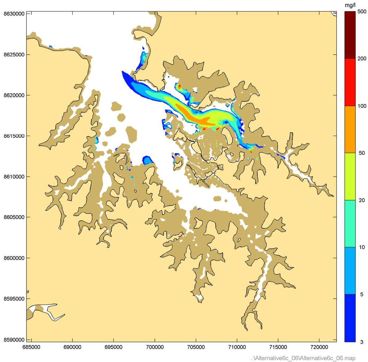
**Figure 65** Instantaneous suspended sediment concentrations during Phase 6 peak ebb – Spring tide (cutter-suction dredger activity)
