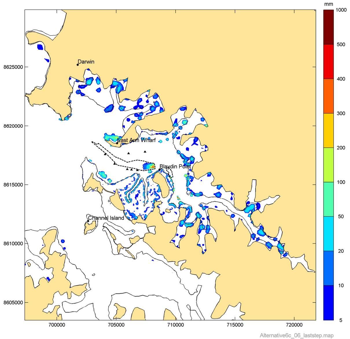
**Figure 89** Simulated depth of fine sediment accretion in the East Arm at the end of Phase 6
