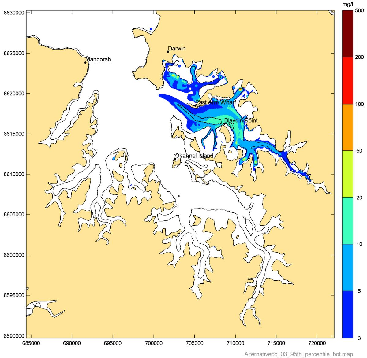
**Figure 31** Simulated 95<sup>th</sup> percentile suspended sediment concentration in the East Arm for Phase 3
