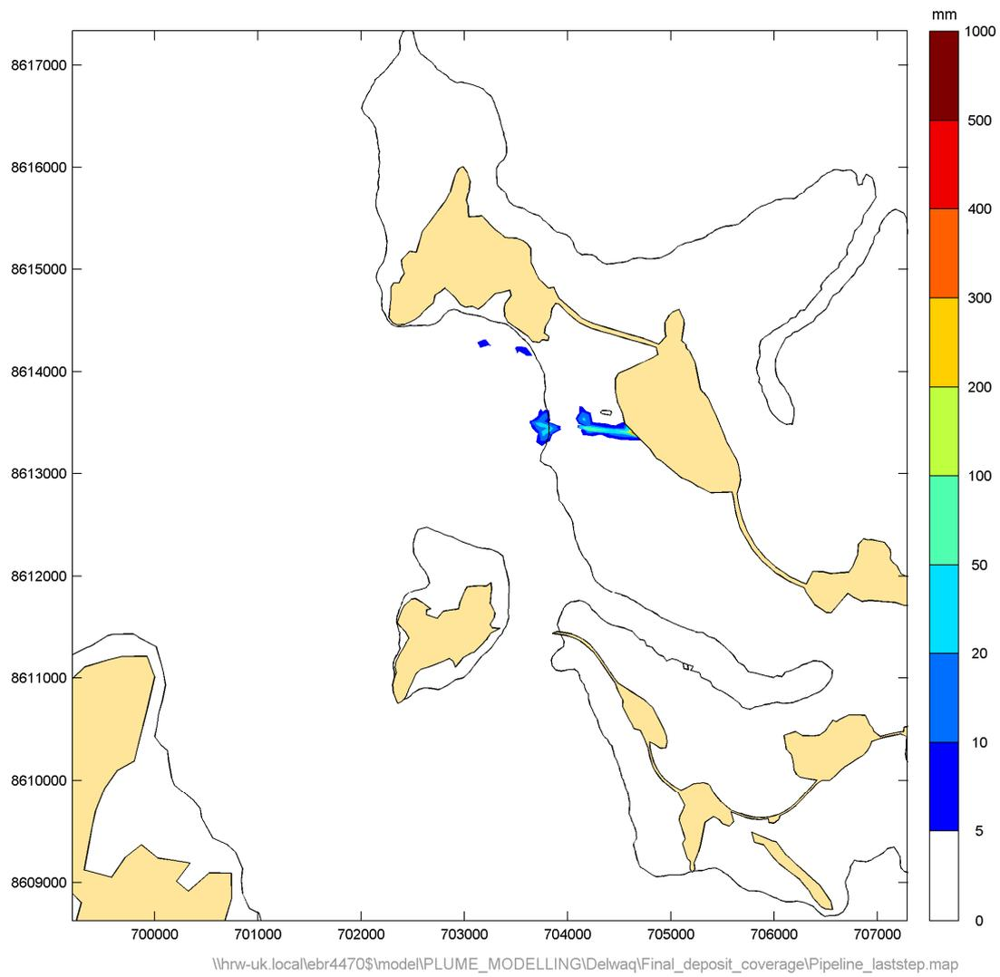
**Figure 17** Simulated depth of accumulation after the completion of the pipeline trench dredge
