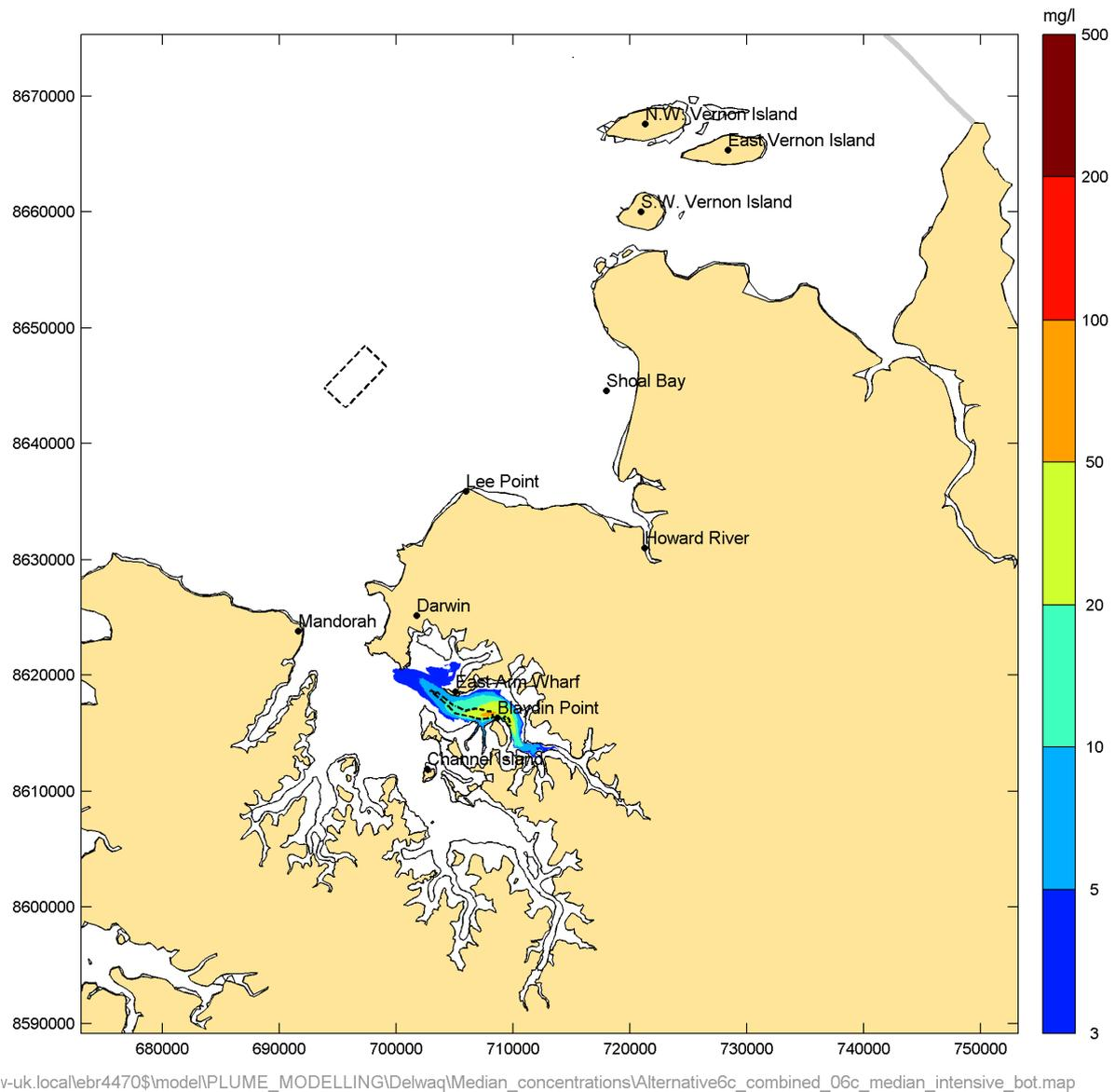
**Figure 100 Simulated median suspended sediment concentrations in the vicinity of Darwin Harbour for all dredging activities during Phase 6 – cutter-suction dredger activity**
