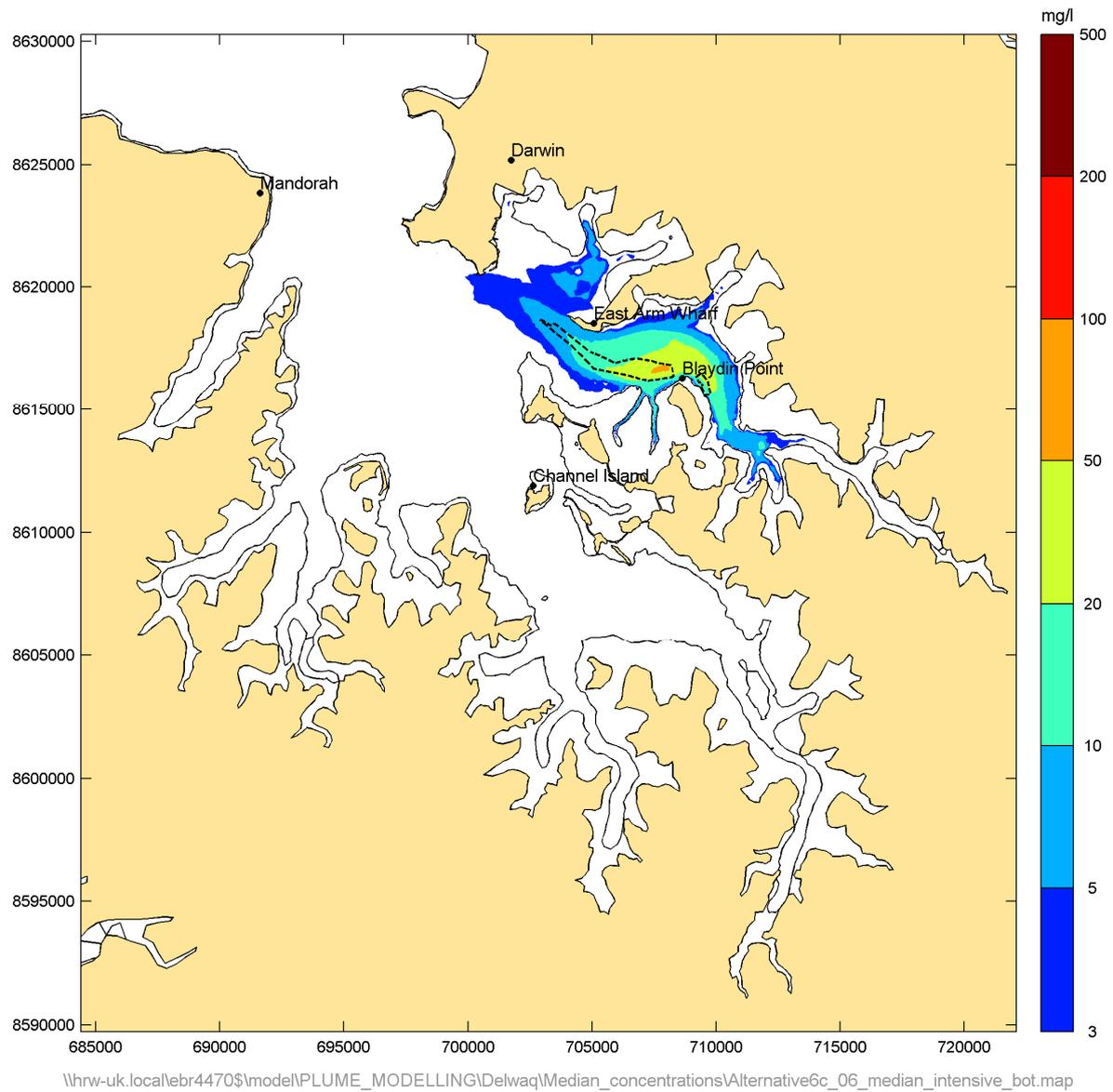
**Figure 24** Simulated median suspended sediment concentration in the East Arm for Phase 6 – cutter-suction dredger activity
