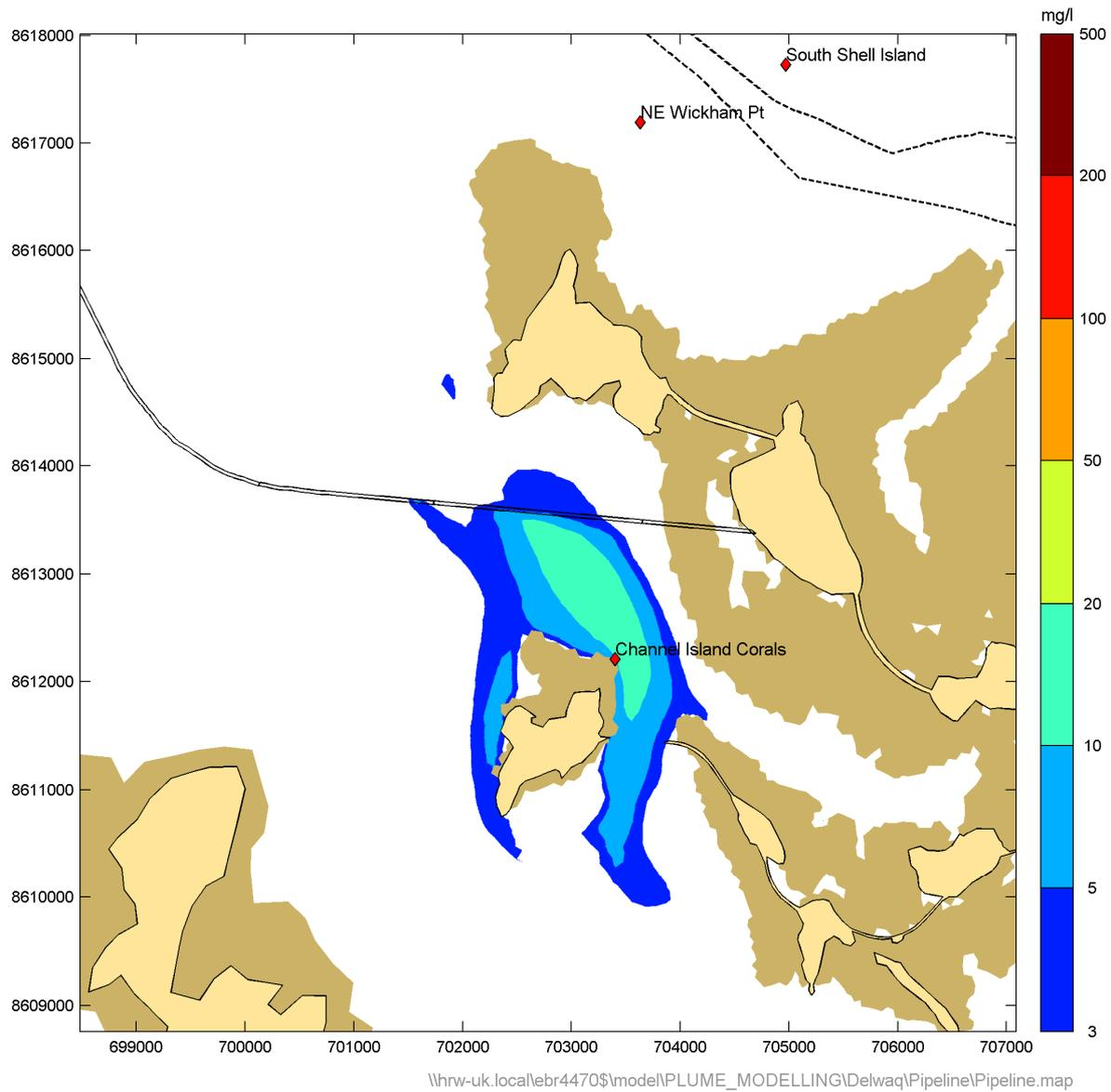
**Figure 16** Colour surface plot of peak concentration at Channel Island during the proposed pipeline trench dredge activity
