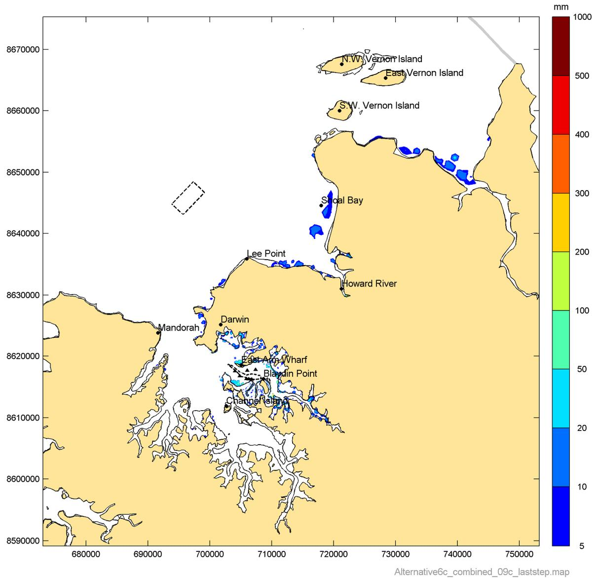
**Figure 124 Simulated depth of fine sediment accretion in the vicinity of Darwin Harbour at the end of Phase 9**
