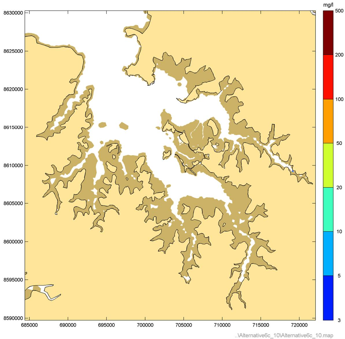
**Figure 80** Instantaneous suspended sediment concentrations during Phase 10 peak ebb – Neap tide
