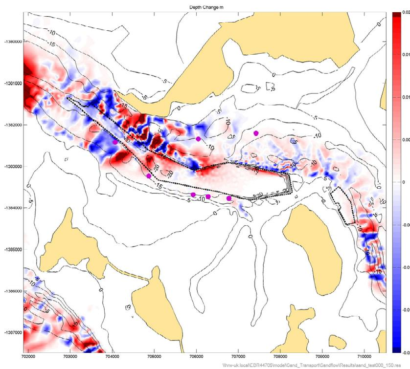
**Figure 133** Indicative areas of net erosion and deposition for spring-neap cycle 150 µm sand under tide-only conditions for postdredge bathymetry
