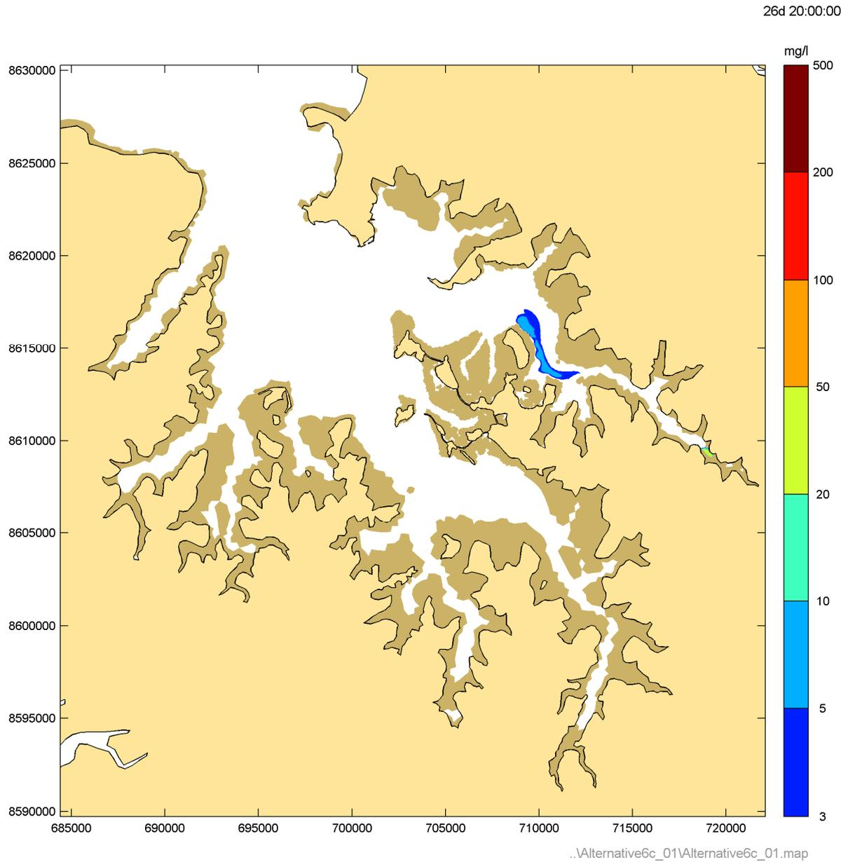
**Figure 41** Instantaneous suspended sediment concentrations during Phase 1 peak flood – Neap tide
