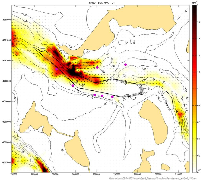
**Figure 132** Net sand transport for spring-neap cycle 150 µm sand under tide-only conditions for postdredge bathymetry
