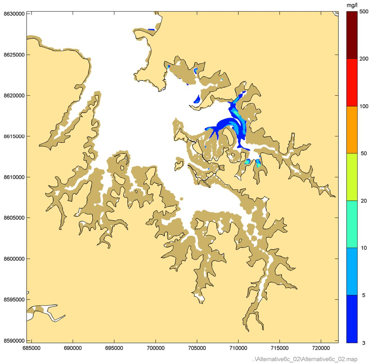
**Figure 47** Instantaneous suspended sediment concentrations during Phase 2 peak flood – spring tide
