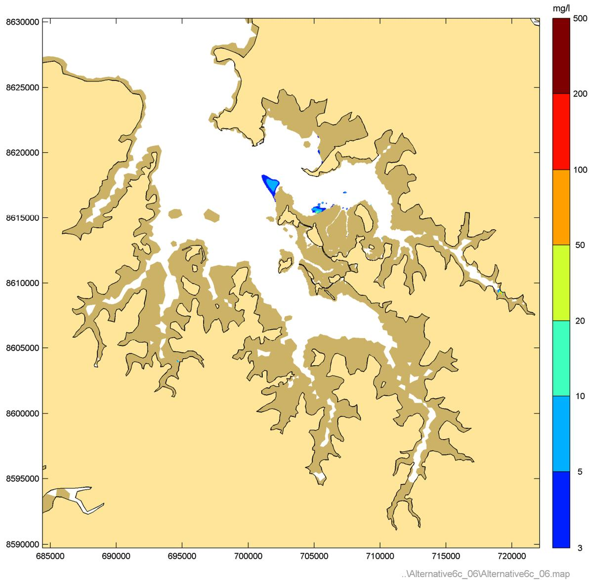
**Figure 60** Instantaneous suspended sediment concentrations during Phase 6 peak ebb – Neap tide
