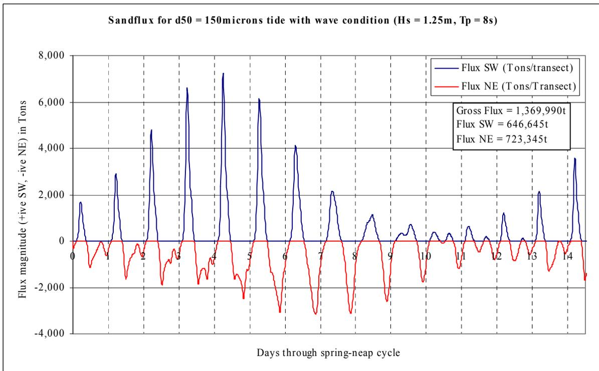
**Figure 142** Potential through tide sandflux magnitudes for spring-neap cycle for tide plus wave conditions and pre-dredge bathymetry at the offshore disposal ground
