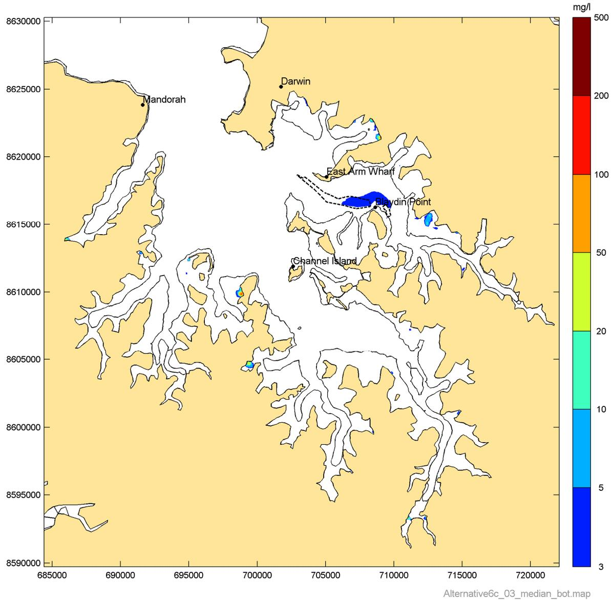
**Figure 20 Simulated median suspended sediment concentration in the East Arm for Phase 3**
