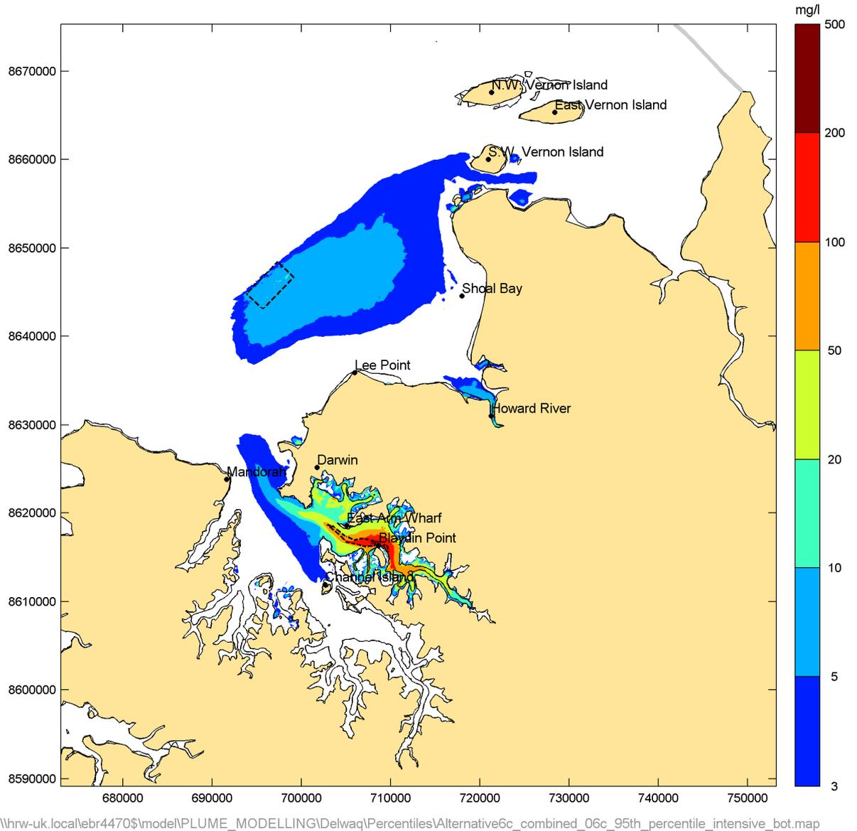
**Figure 111 Simulated 95<sup>th</sup> percentile suspended sediment concentrations in the vicinity of Darwin Harbour for all dredging activities during Phase 6 – cutter-suction dredger activity**
