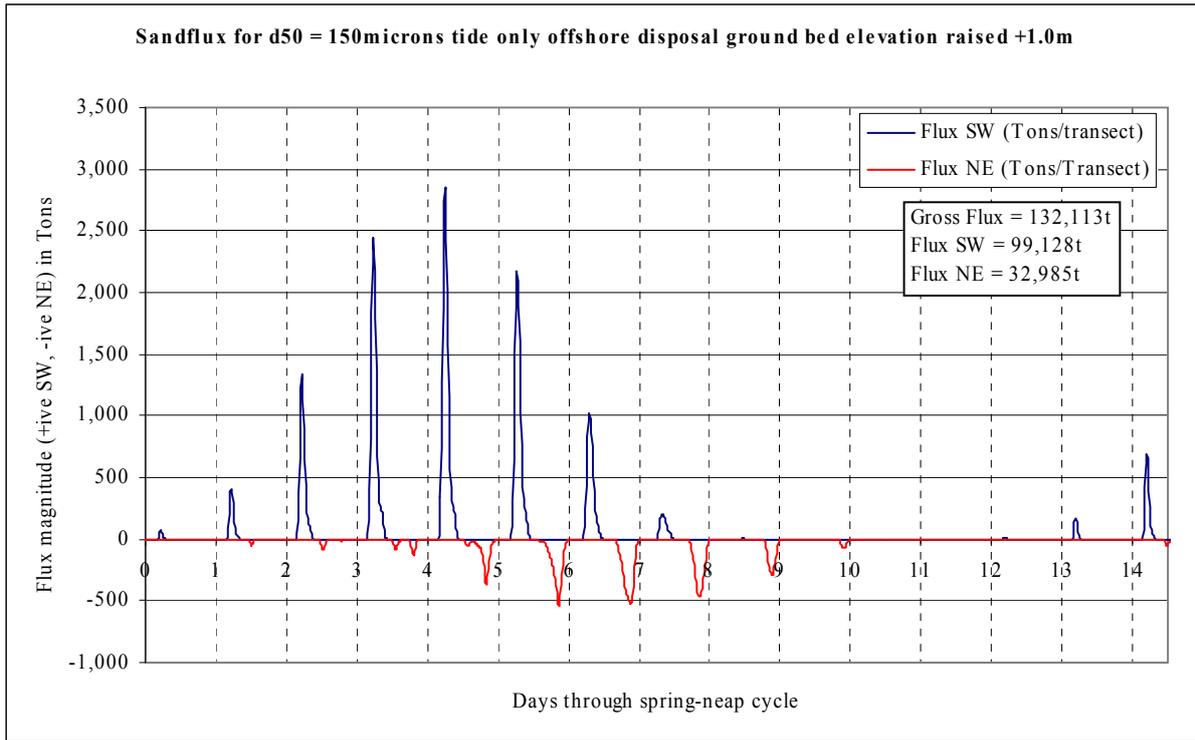
**Figure 147 Potential through tide sandflux magnitudes for spring-neap cycle for tide-only conditions and post-dredge bathymetry at the offshore disposal ground**
