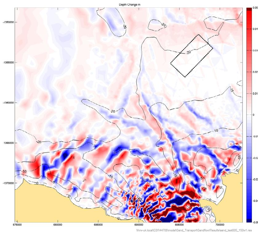
**Figure 140** Indicative areas of net erosion and deposition for spring-neap cycle 150 µm sand under tide plus wave conditions for pre-dredge bathymetry
