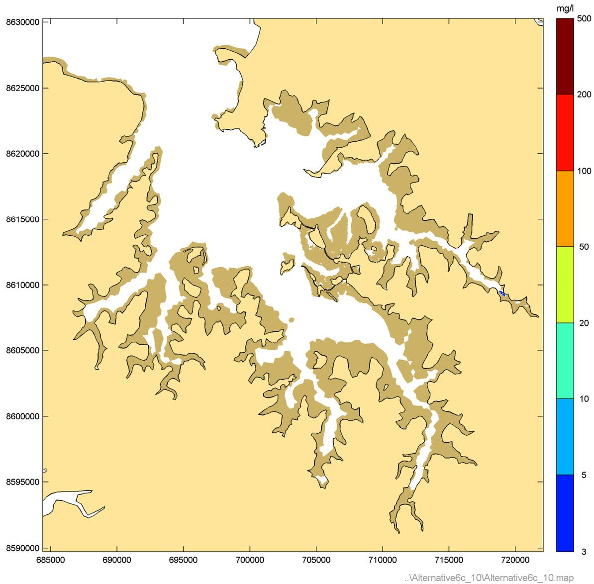
**Figure 81** Instantaneous suspended sediment concentrations during Phase 10 peak flood – Neap tide
