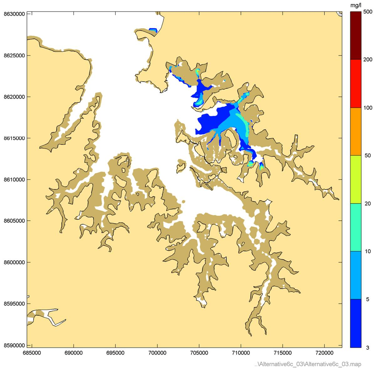
**Figure 51** Instantaneous suspended sediment concentrations during Phase 3 peak flood – spring tide
