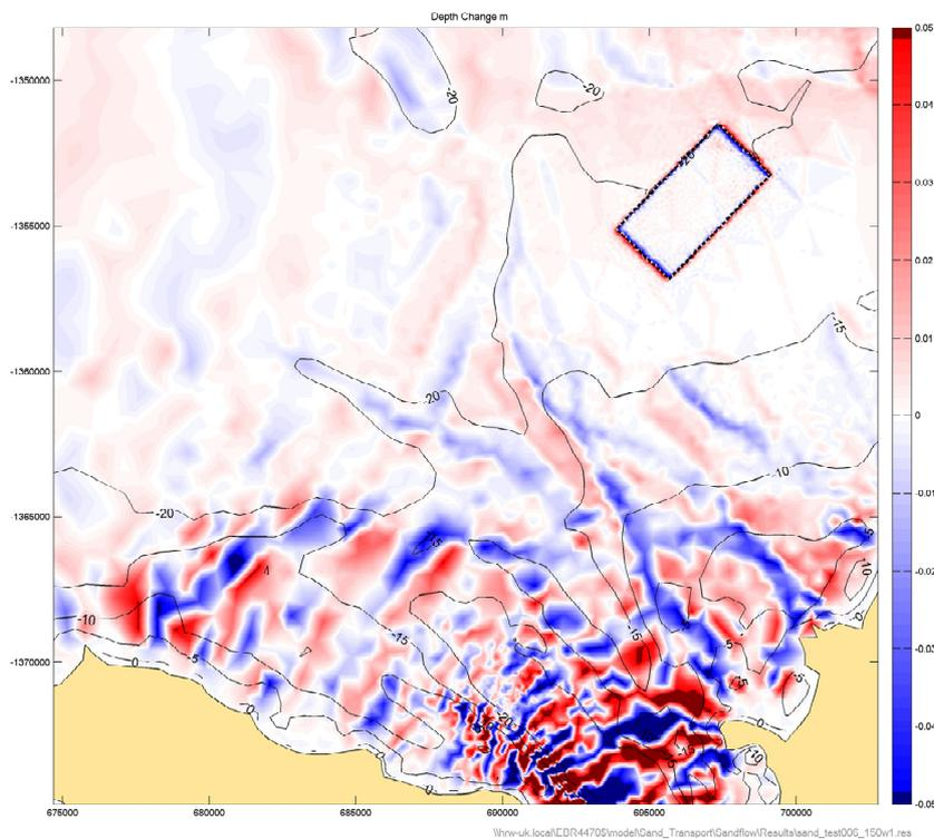
**Figure 146** Indicative areas of net erosion and deposition for spring-neap cycle 150 µm sand under tide plus wave conditions for post-dredge bathymetry (offshore disposal ground +1.0m)
