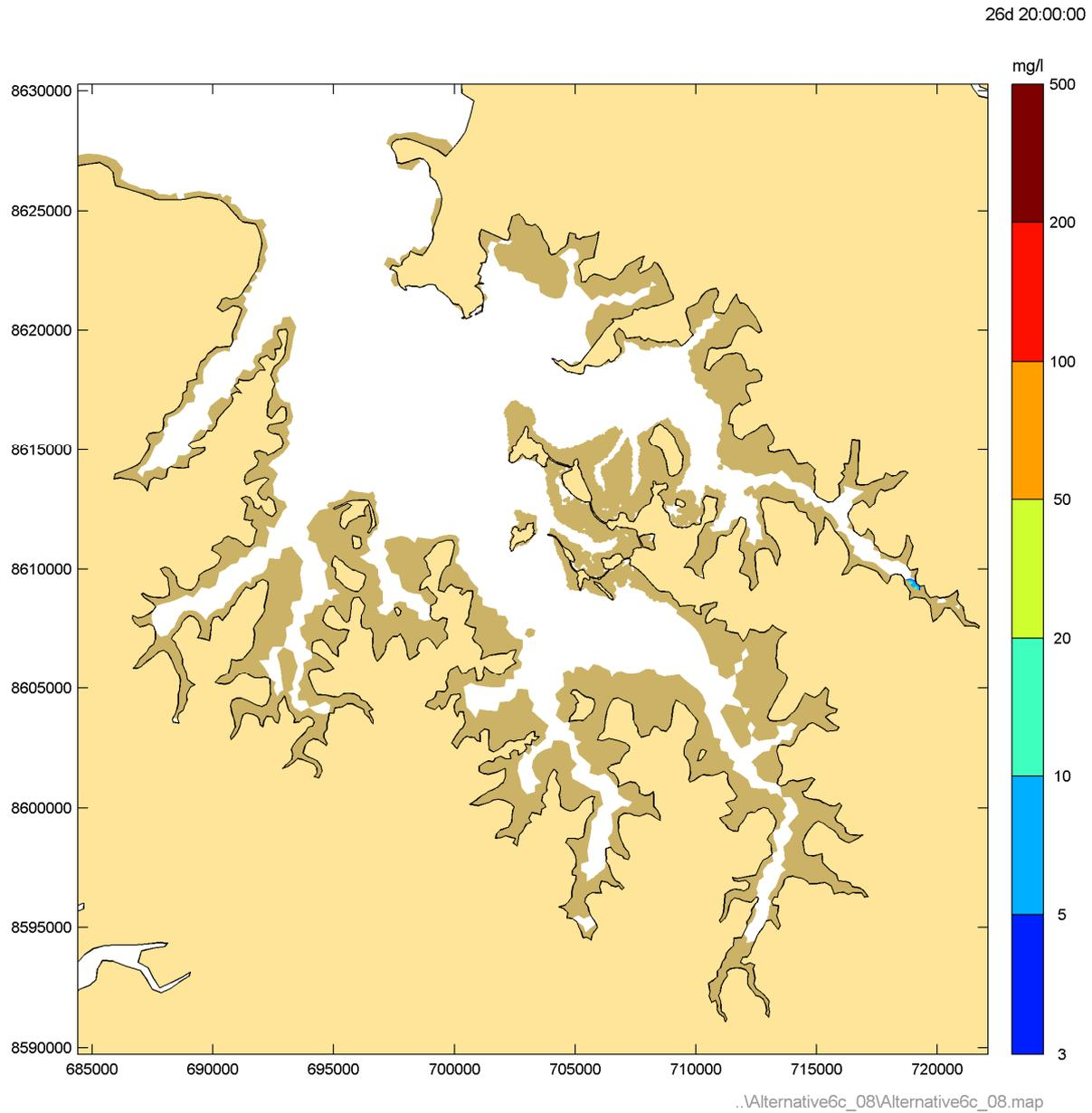
**Figure 73** Instantaneous suspended sediment concentrations during Phase 8 peak flood – Neap tide
