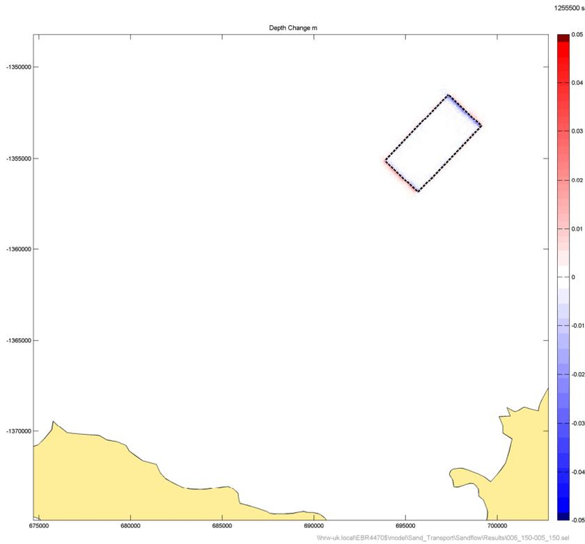
**Figure 149** Difference in potential area and magnitude of deposition and erosion at the proposed offshore disposal ground under tide only conditions
