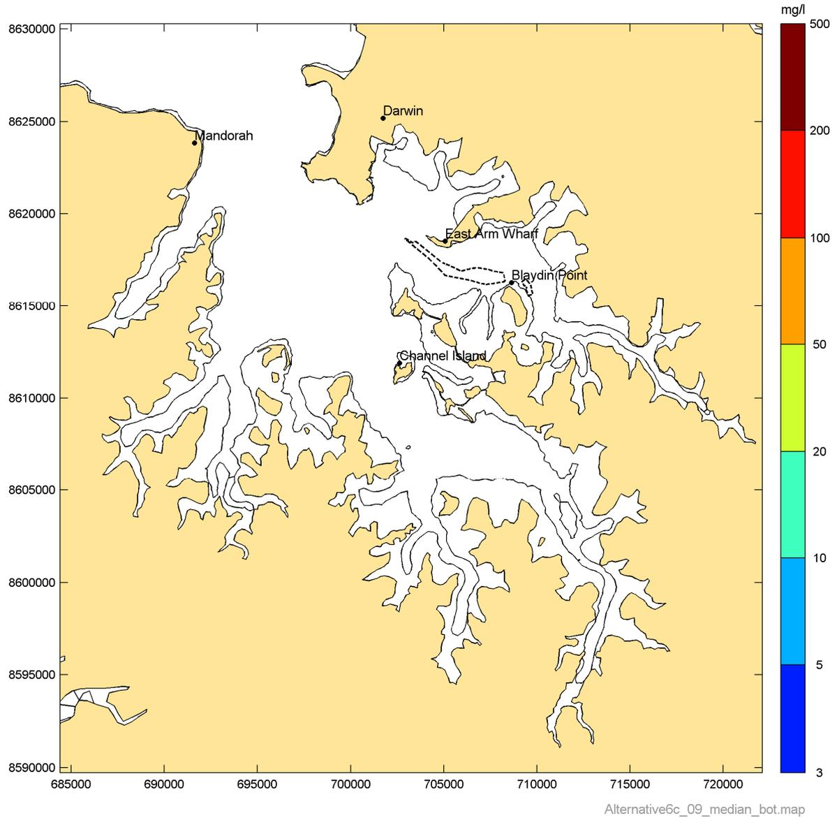
**Figure 27 Simulated median suspended sediment concentration in the East Arm for Phase 9**
