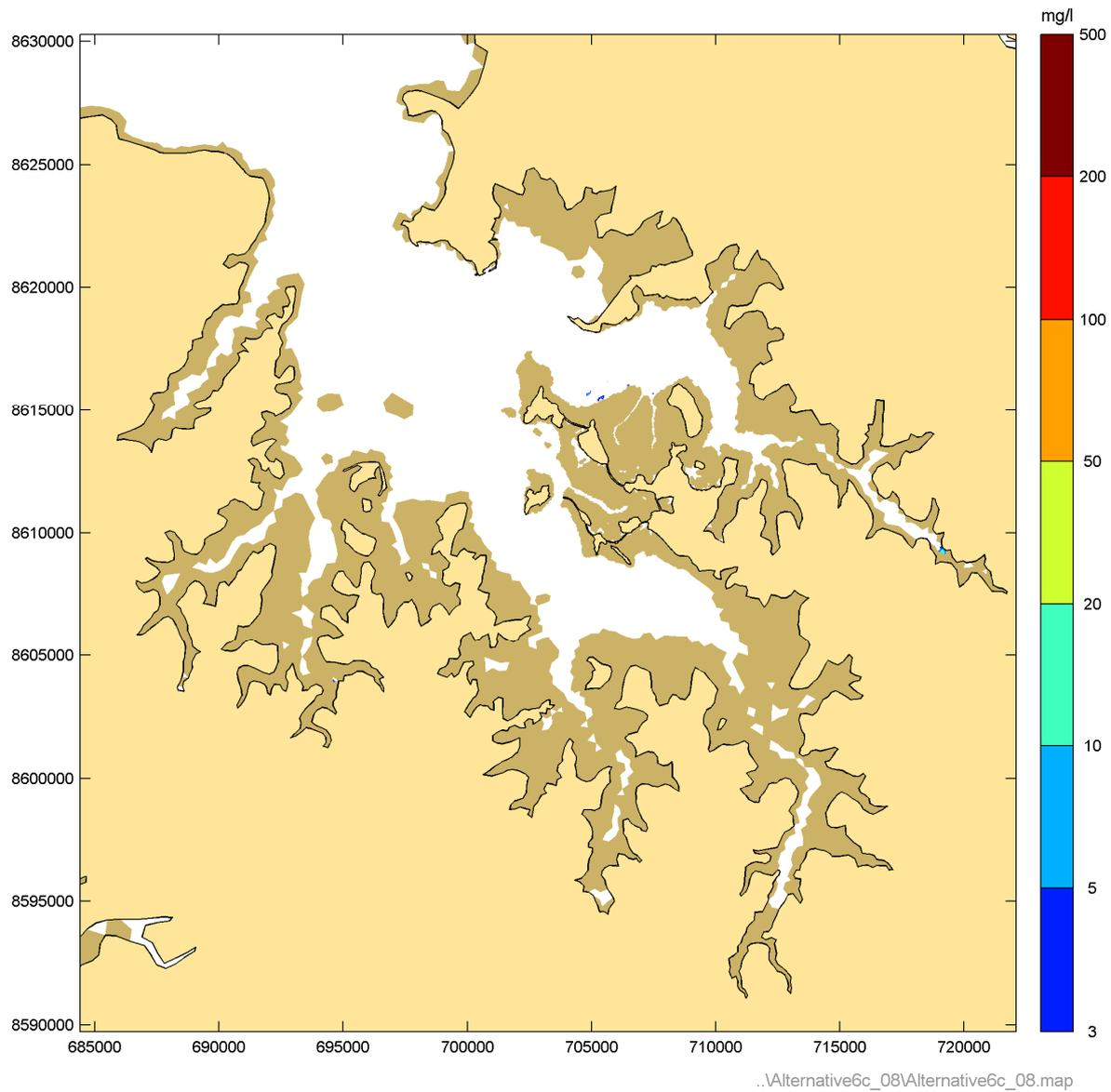
**Figure 72** Instantaneous suspended sediment concentrations during Phase 8 peak ebb – Neap tide
