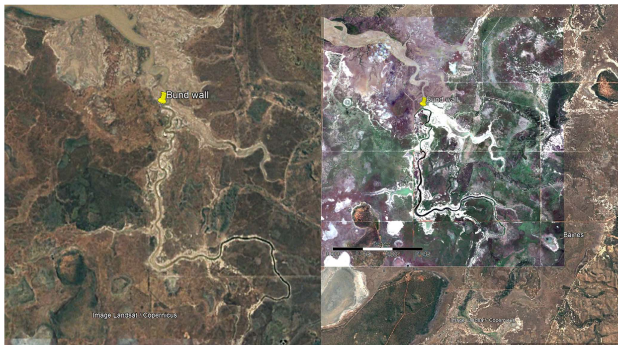
Figure 13. Legune Station floodplain country with infrastructure development in blue carbon communities. The LH panel is from 2001 (Google Earth composite) prior to a track and bund wall construction in 2002/2003. The RH panel is a higher resolution Sentinel-2 image from 2019 with the bund wall potentially altering tidal ingress and ponding of river flow that may be associated with high methane emission. Such a site could be assessed in collaboration with land managers in Phase 2 of this project.
