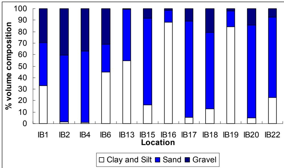
Figure 5-7 Distribution of particle sizes in sediments at offshore locations in September 2005. Source: RPS (2007a)
