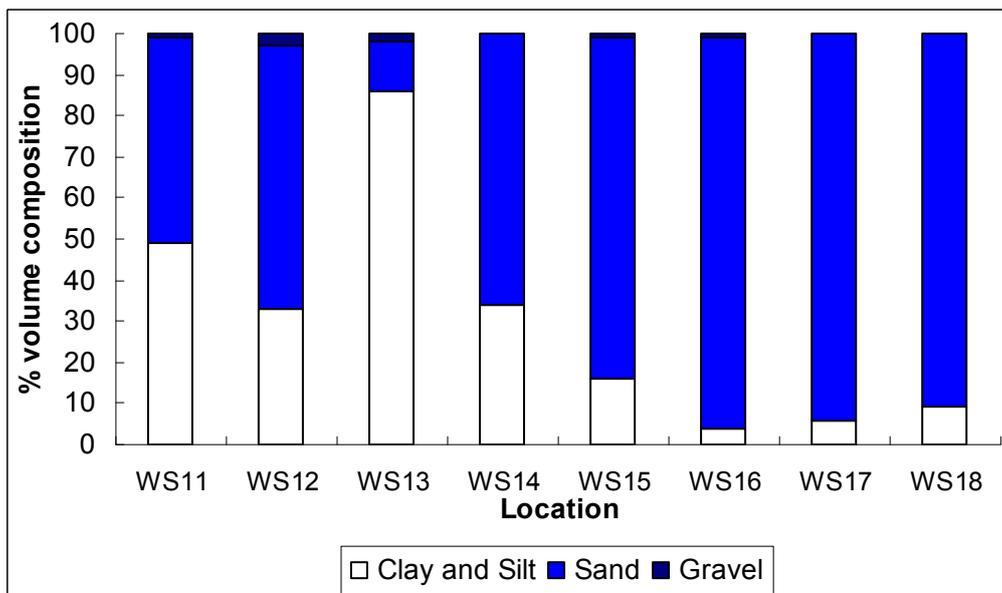
Figure 5-8 Distribution of particle sizes in sediments at offshore locations in May 2007. Source: RPS (2007a)
