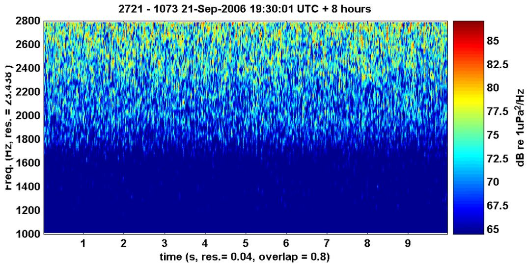
Figure 8-5 Spectrogram of offshore high-frequency fish chorus.
