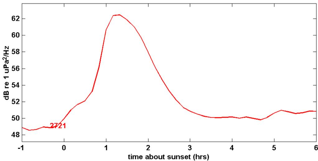
Figure 8-6 Evening fish chorus from the offshore site, with time zeroed to local sunset and the chorus level in the 2 kHz  $\frac{1}{3}$  octave averaged over the full recording period. Source: RPS (2007b)
