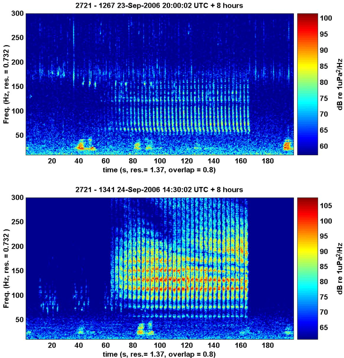
**Figure 6-27** Spectrograms of variants of possible Antarctic minke whale signals (60–170 secs each plot) recorded at the offshore logger on 23–24 September 2006. Weaker humpback signals are evident in the background (energy over 50–200Hz) and an unidentified great whale signal is evident over 25–50Hz. Source: McCauley (2009)
