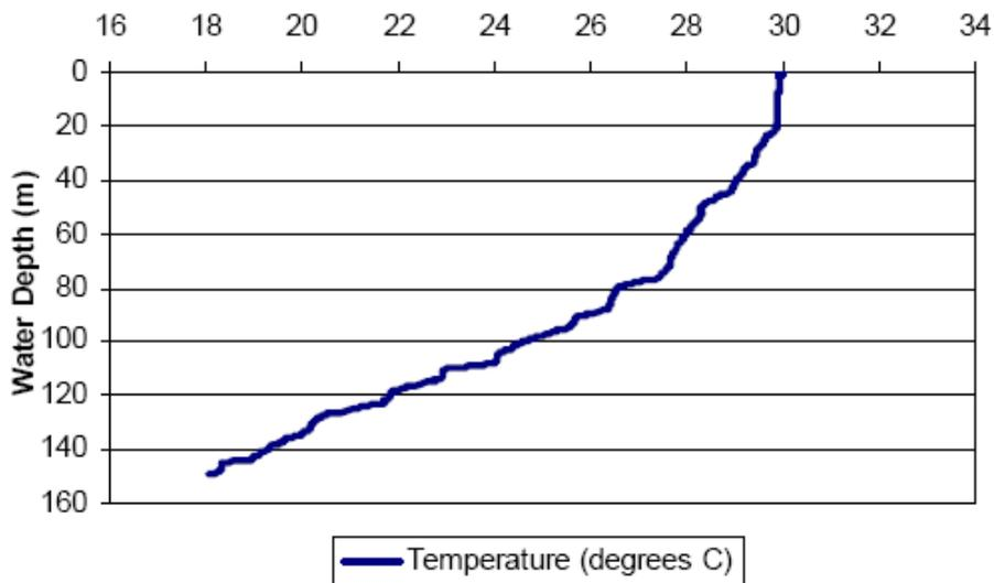
Figure 5-4 Vertical water column profile at Site WQ13, May 2007.
