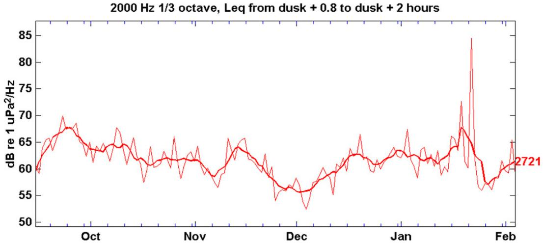
**Figure 8-7 Seasonal pattern in 2 kHz, 1/3 octave averaged over 0.8 to 2 hrs post dusk each evening as an indicator of changes in fish chorus level. Source: RPS (2007b)**
