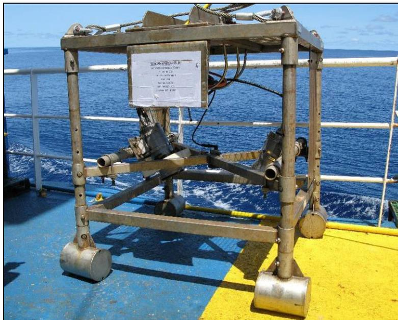
**Figure 4-2** Drop camera set-up used for the survey
