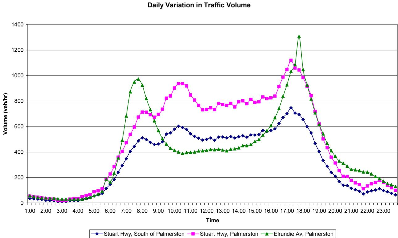
Existing midblock daily traffic volumes are shown in Figure 4-2 while Figure 4-3 and Figure 4-4 show the AM (7:15am – 8:15am) and PM peak hour (4:30pm – 5:30pm) turning movement volumes at intersections, including the percentage of commercial vehicles.
